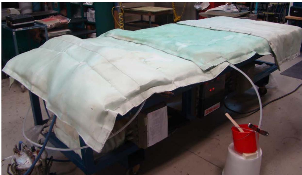
Figure 3. Heat table with insulating blankets placed over the laminates during the curing cycle.
