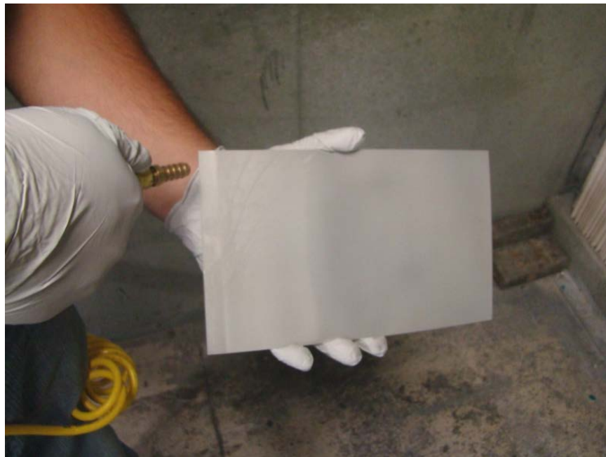
Figure 7. Image of the high-pressure nitrogen gas stream-drying process to the 2024-T3 aluminum alloy flexible adherend.
