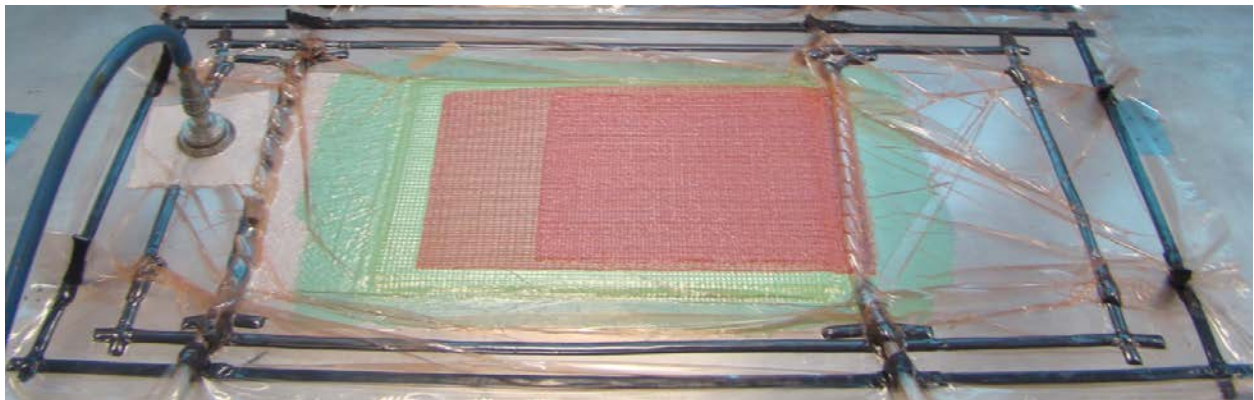
Figure 2. Vacuum-bagged laminate during the debulk process.
