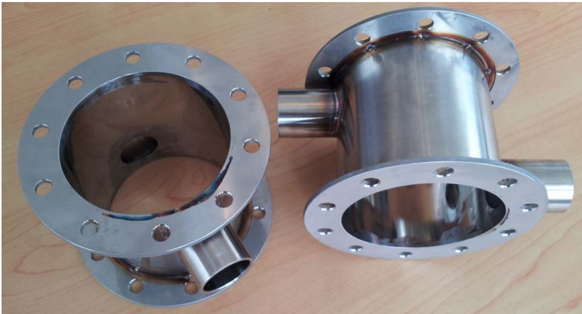
Figure 10. Completed initial reaction vessel; three inch diameter and three inch length main pipe, one inch diameter flow through pipes all made of sanitary, food-grade finish 316 stainless steel pipe, final polishing via electro-polish process.
