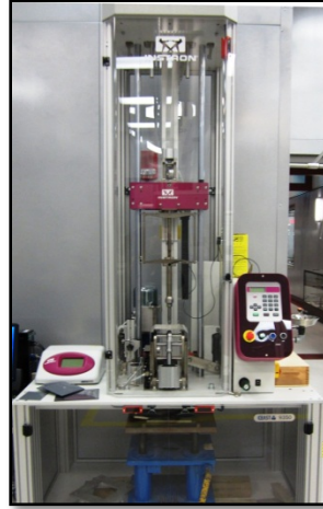
Figure 8. Impact Panel Test Setup
