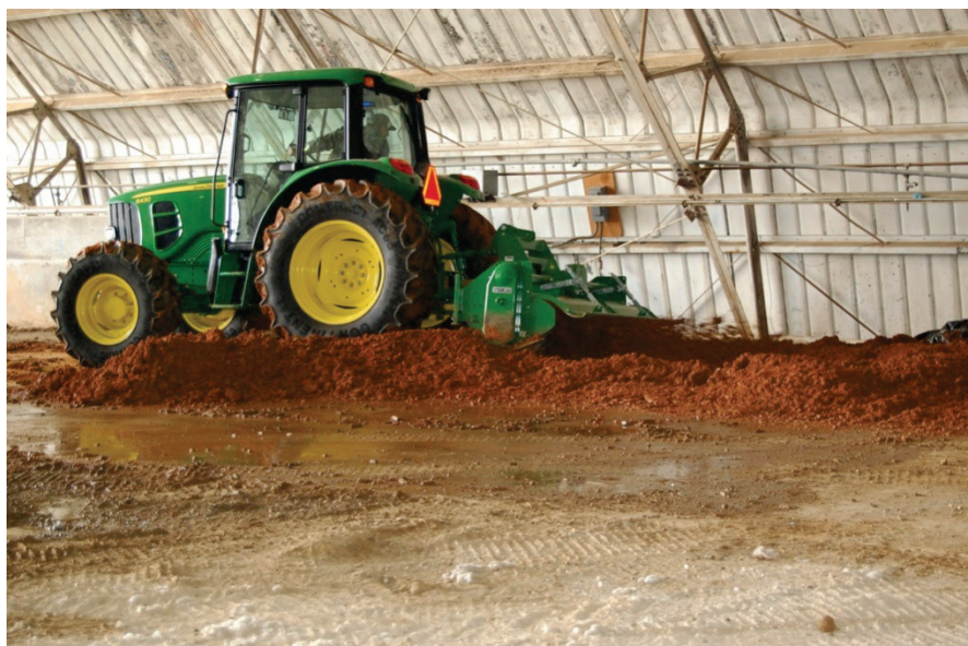
Figure 10. Tiller used to loosen the soil during soil preparation.
