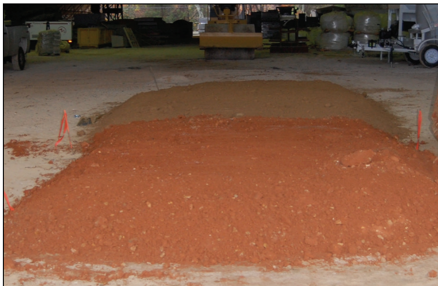
Figure 8. Test Strip 1 consisting of silt in the South Test Item (back) and clay-gravel in the North Test Item (front).
