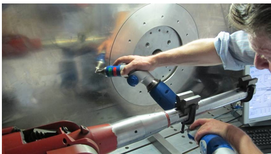
Figure 13: CMM measuring the inner sidewall reference plane
