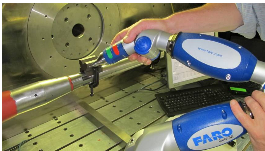
Figure 12: CMM measuring the rear 'V' block side face
