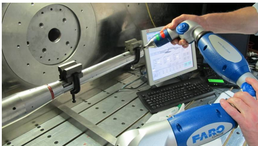
Figure 11: CMM measuring the front 'V' block side face
