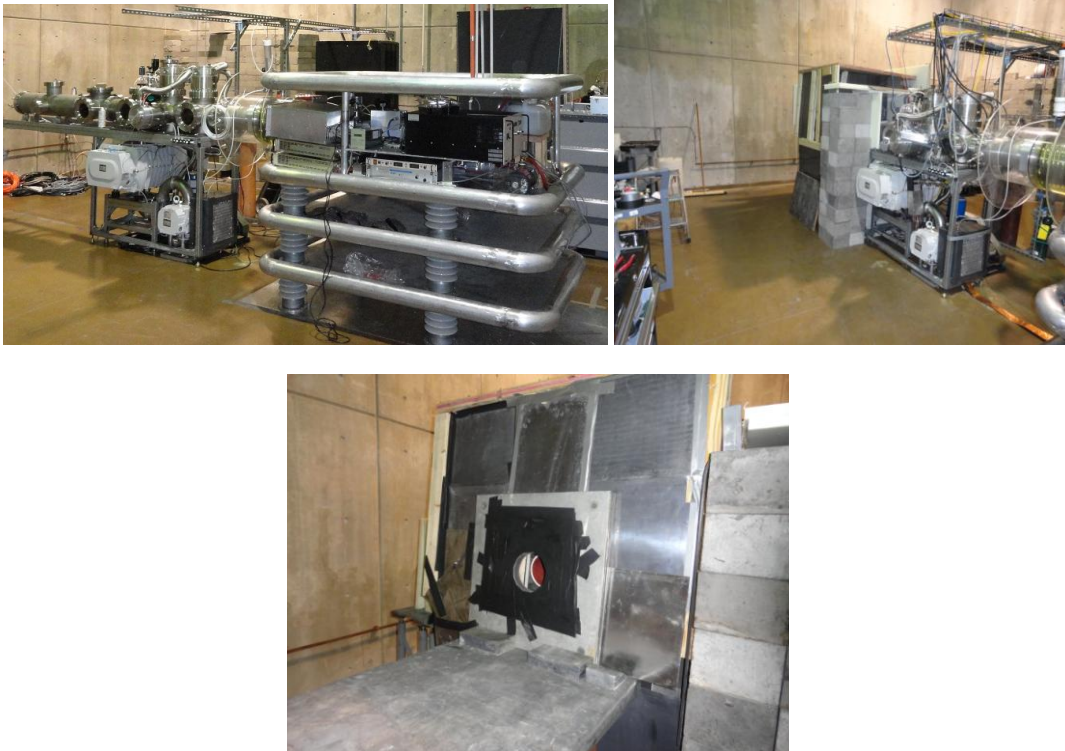
Figure 7: The initial setup of the PNL neutron generator system at ARDEC, without moderator (top left), with added graphite, concrete, and boron shielding (top right), and the first design of the beam port (bottom).
