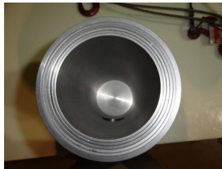
Figure 1: Low-carbon steel insert used to slow the high-energy D-T neutrons over a shortened distance.
