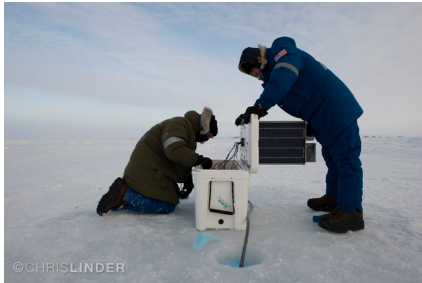
Figure 3: Two aerospace engineering students from the U.S. Naval Academy attempt to troubleshoot the Arctic Observing Platform IceKid2A while on the ice off Barrow, AK. The design and build of this platform was the midshipmens senior capstone design project. IK2A is solar powered, and capable of relaying under ice acoustic data in near real time via satellite communications.
