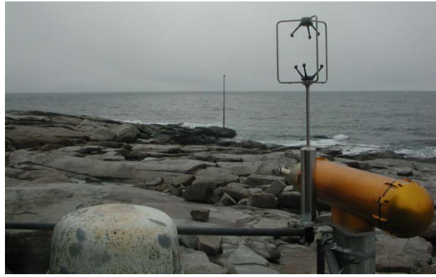
Figure 3. Cloud imaging probe and its associated sonic anemometer/thermometer mounted on the foghorn platform on Mt. Desert Rock.
