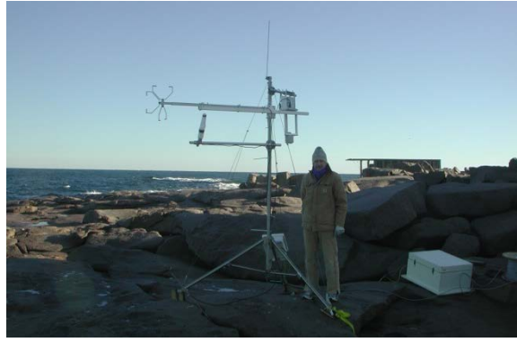
Figure 2. Mast on which we measured mean meteorological quantities and the turbulent fluxes of momentum and sensible heat.
