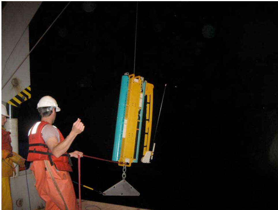
Figure 1. A Macro WW being deployed in the Dynamo experiment.
