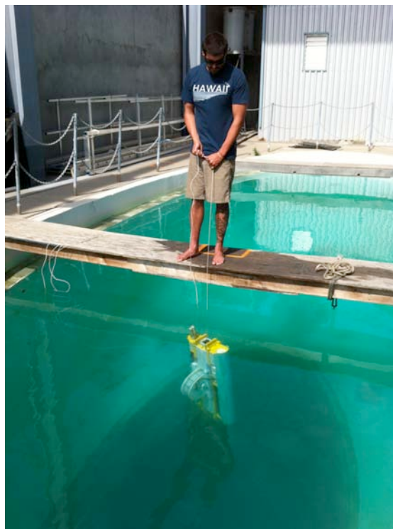
Figure 2. A Livewire power-generating float being tested at SIO. This first-generation device produces nearly 1 W in calm conditions. It is hoped that future devices will produce 1-5 W in typical oceanic conditions.
