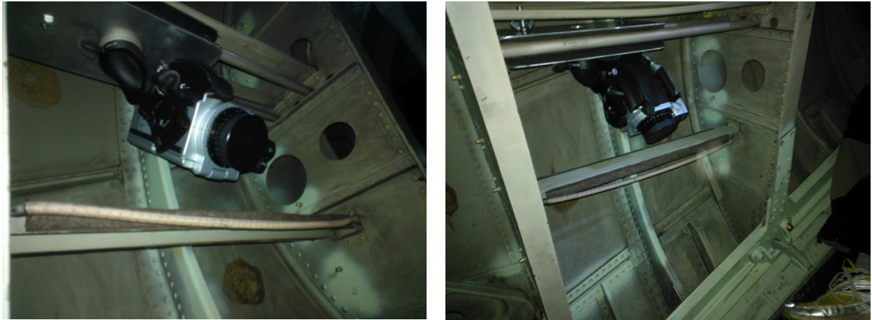
Figure 1. Two views of the test mounting of the handheld IR camera adjacent to the rear cargo door. The camera view of the ocean-ice surface is near nadir (straight down) when the cargo door is open for deployment of instruments during flight.
