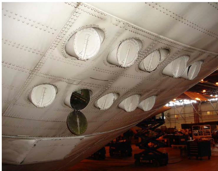
Flare tubes on the rear door of a C-130 aircraft where the CULPIS-X instrument package will be installed.
