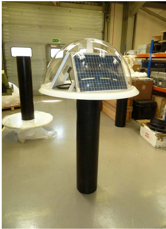
Figure 1: Prototype wavebuoy in the workshops at BAS. The finished buoy has a large flotation collar below the solar panel deck.
