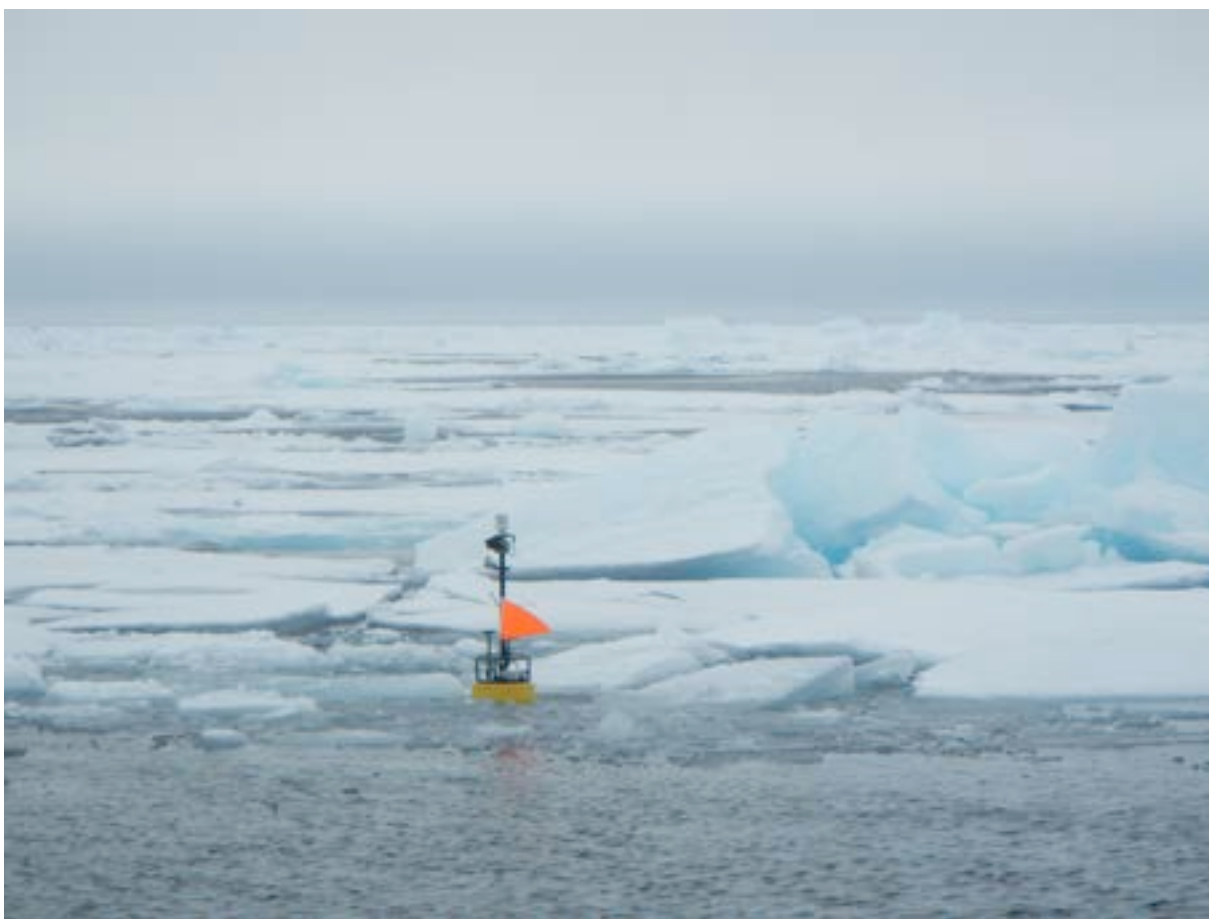
Figure 1. SWIFT buoy deployed from USCGC Healy in Sep 2013 for ice testing prior to 2014 field experiment.
