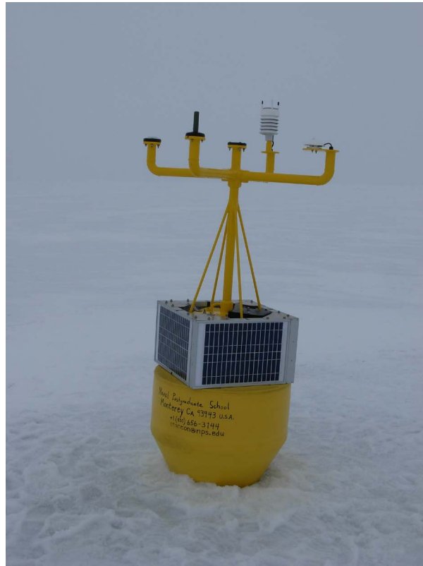
Figure 1. A Met-package AOFB deployed in the Beaufort Sea.
