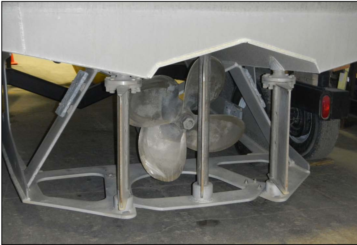
Figure 14. ACS boat propeller shroud.
