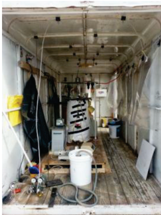
Figure 17. Set up of the anaerobic digester at LWI. Tedlar bags to collect gas on the upper right of the photograph, the one at the very end is expanded due to collected gas.
