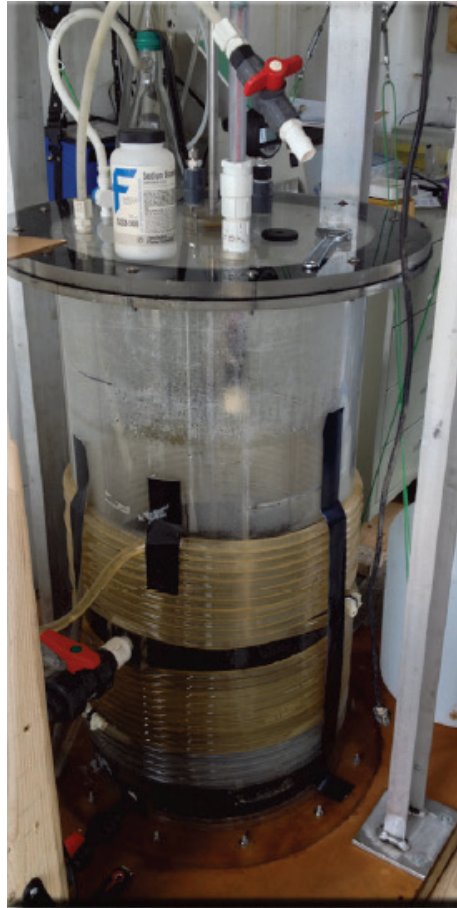
Figure 18. Bioreactor with insulation removed showing coiled tubing that was part of the temperature control system.
