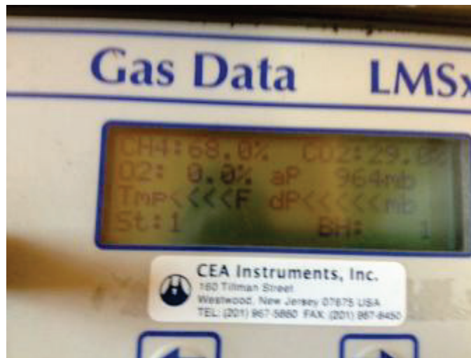
Figure 38. Gas meter reading on biogas stored in Tedlar storage bag showing methane content at 68%.
