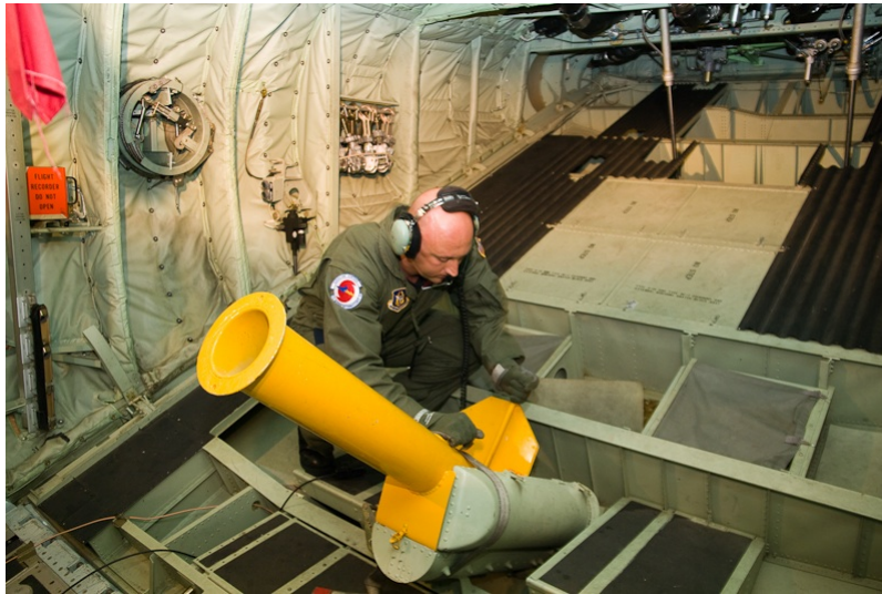
Figure 1. Flare Tube adaptor designed to convert a C-130 flare-tube into a device that allows deployment of drop sondes and Sonobuoy Type -A devices.
