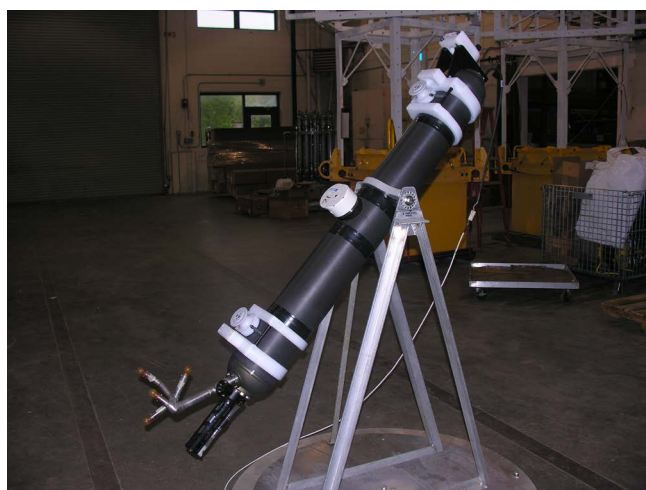
Figure 3. Photograph of an ITP-V in the jig during a test spin to quantify sensor relative orientations. (Actual spin tests are conducted outside in an area free from artificial magnetic fields.)
