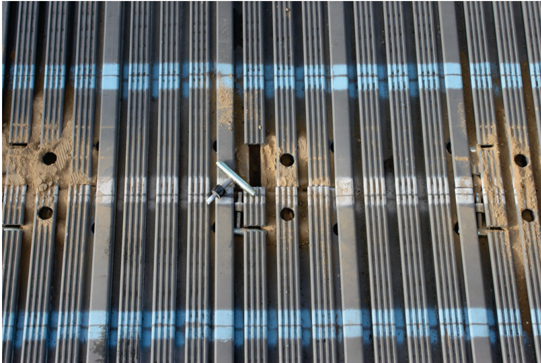
Figure 29. Broken mat panel after 112 passes on the 25-50 CBR section.
