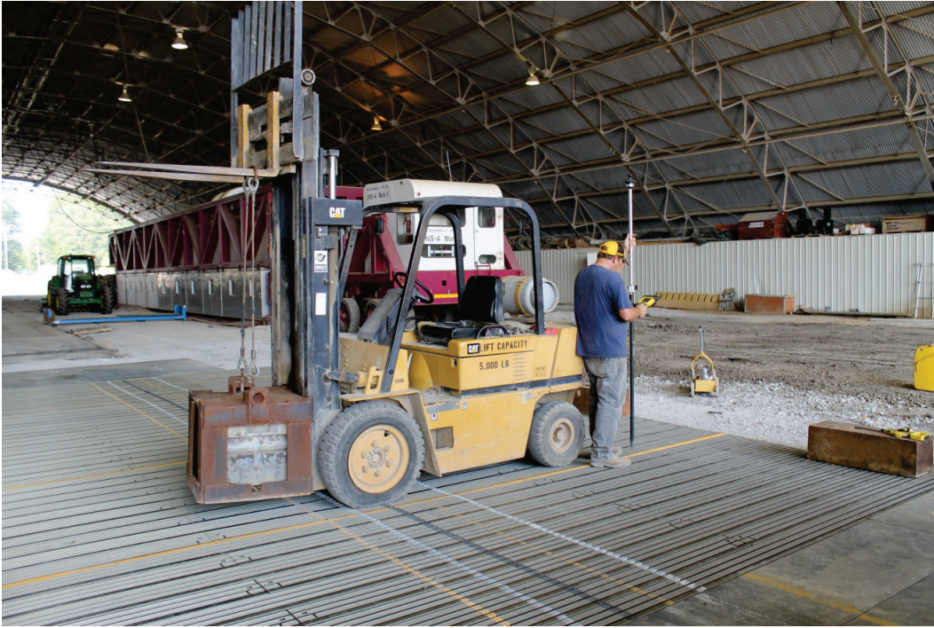
Figure 27. Typical loaded cross-section data collection.
