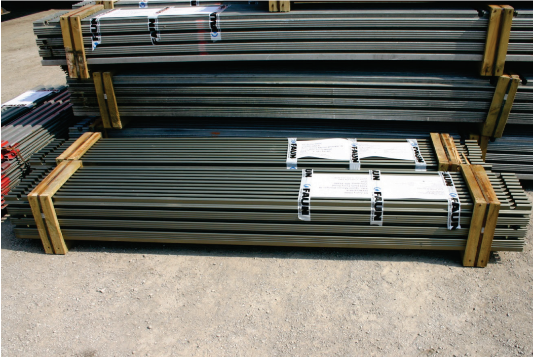
Figure 4. MLC-70 Trackway panels.
