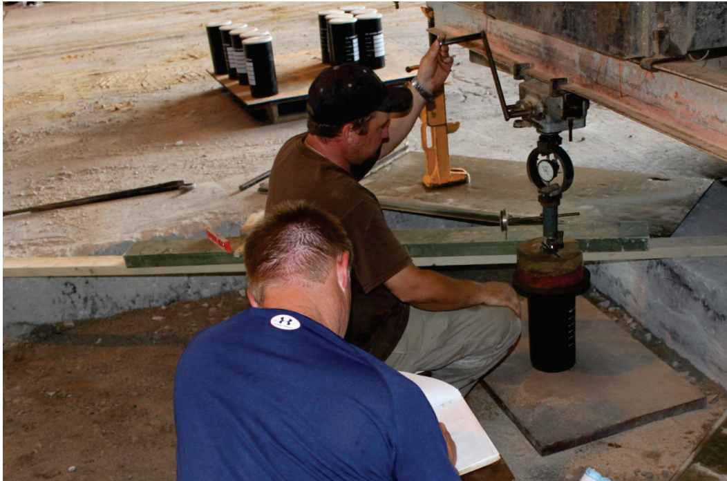
Figure 8. Conducting field CBR test in 6-in. cylinder molds.
