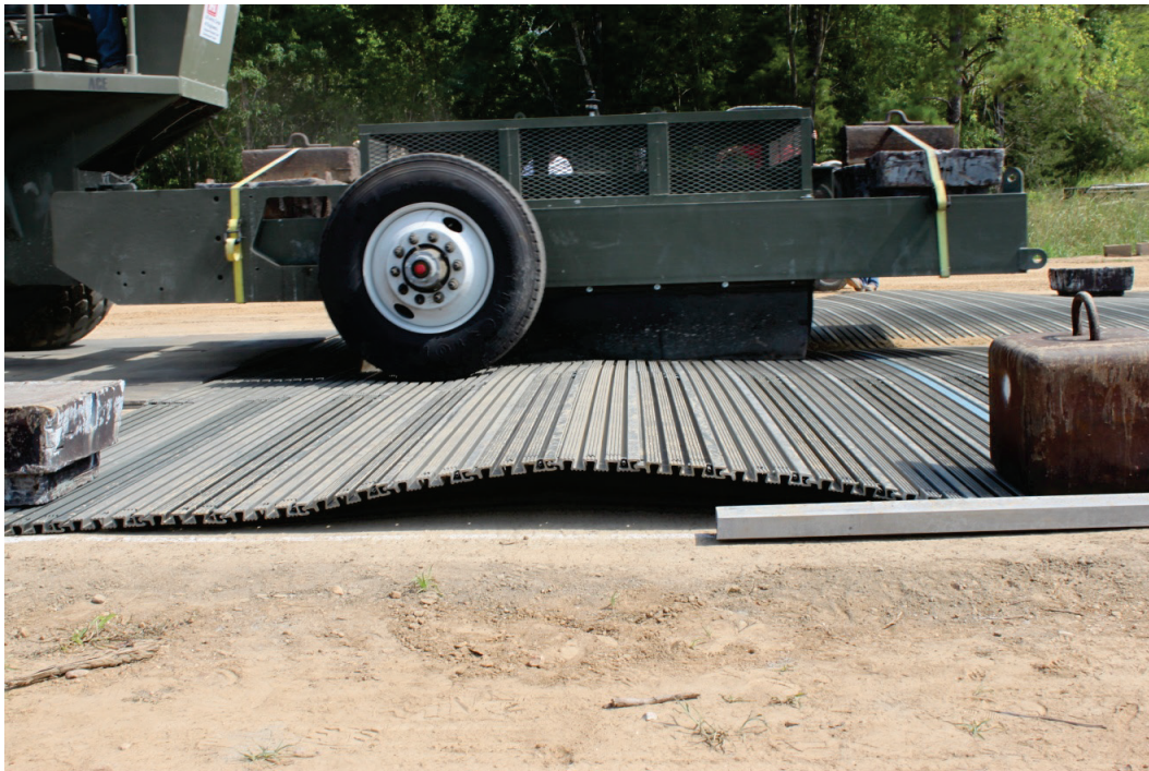
Figure 30. Excessive rutting and bow-wave formation after 240 passes near A1 on the 25-50 CBR section.
