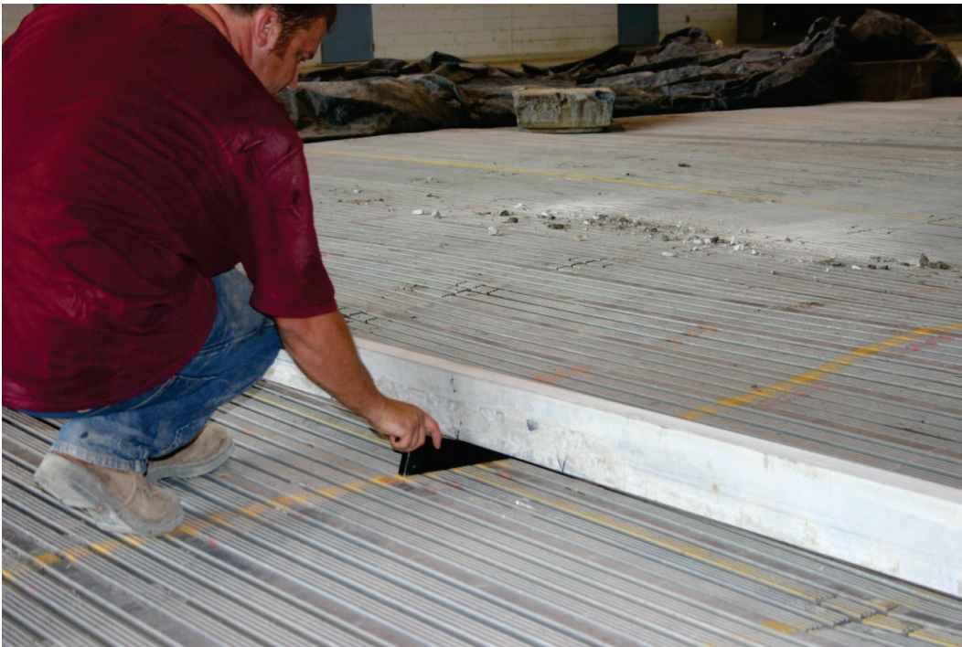
Figure 28. Typical unloaded rut depth measurements.
