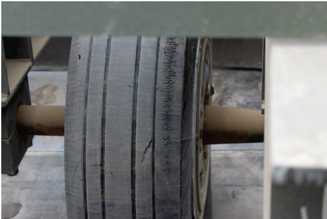
Figure 32. Tire damage after trafficking 25-50 CBR test section.
