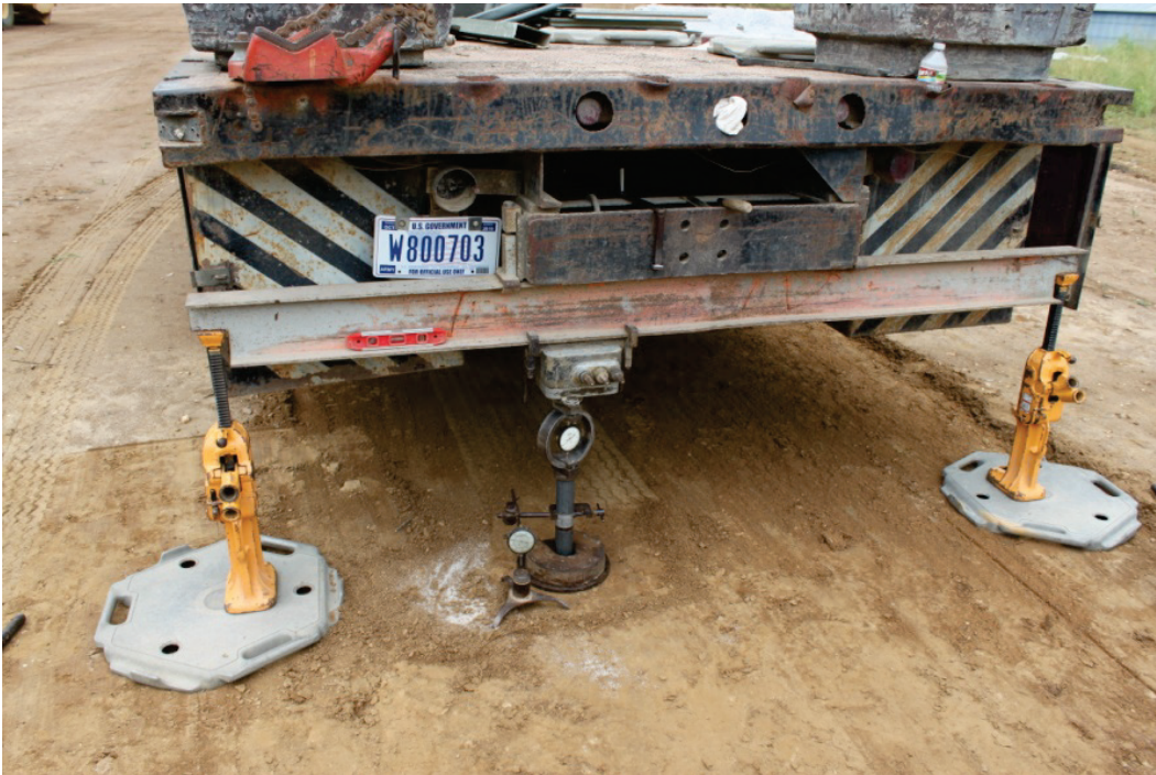
Figure 12. Field CBR test.
