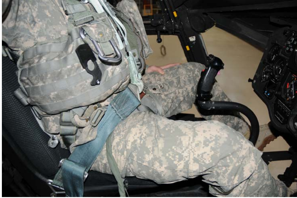
Figure 9. Pressure on collecting tube due to restraint harness design in left pilot seat of CH-47.
