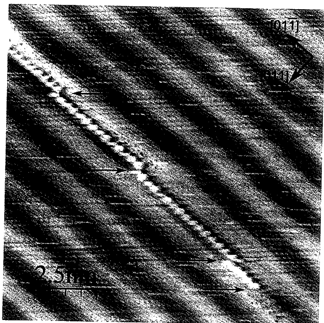
FIG. 7. (Color online) STM image of a gold adatom, produced by neon sputtering, moved over the reconstructed Au(100) by the scanning tip. Scanning at 100 K under manipulation conditions, at 20 nA and 12 mV, is along the horizontal, from the bottom to the top. The adatom moves over an appreciable length along one [01\bar{1}] atom row, until as indicated by arrows, it jumps to an adjacent one, where it continues its movement. A subsequent STM image does not show the atom.
