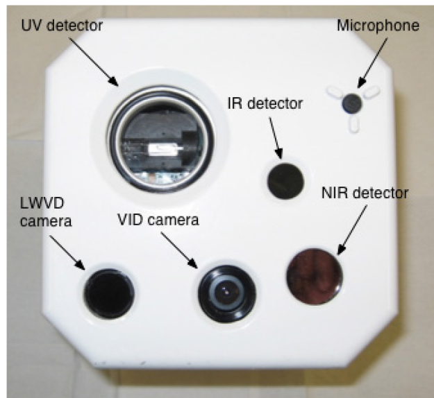
Figure 2 - Sensor head unit of the Canadian Demonstrator Prototype – Volume Sensor Sensor.
