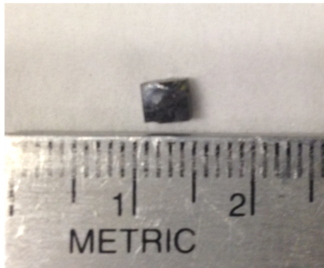
Figure 1.4: Heavily-doped thorium oxide crystal, 041 TU, with uranium mass concentration of 22.7% before chemical cleaning. Mass pre-cleaning: 0.341 g.
