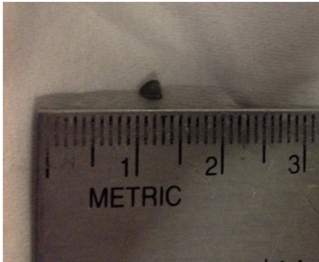
Figure 1.2: Lightly-doped \text{U}:\text{ThO}_2 crystal, 003 TU, with uranium mass concentration of 1% before chemical cleaning. Pre-cleaning mass: 0.0027 g.
