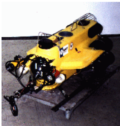
Figure 2. A US Navy self-propelled remotely operated vehicle able to take video and pictures. (Photograph from http://www.navy.mil/navydata/nav_legacy.asp?id=291 courtesy of Oceaneering Technologies, Upper Marlboro, MD.) 29
