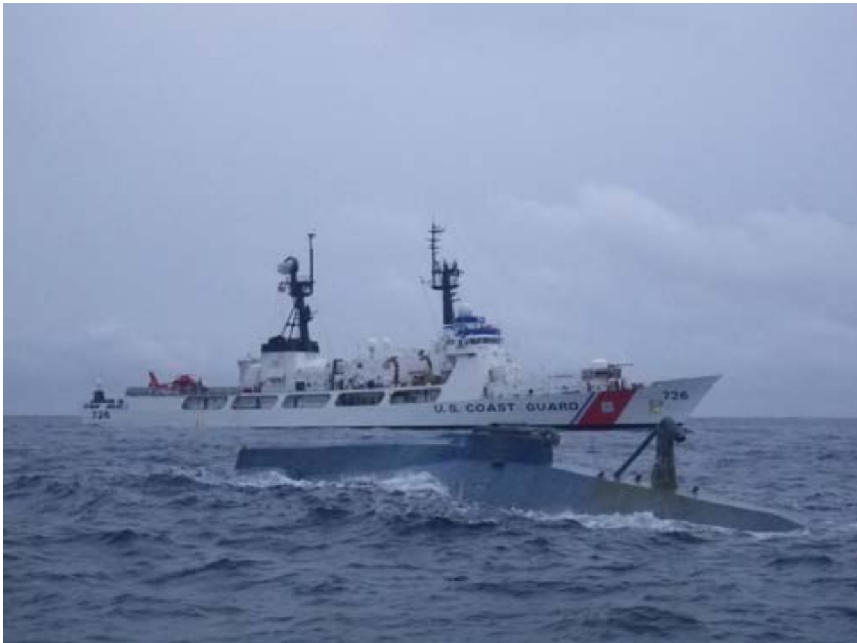
Figure 5. Pictures of 35-foot self-propelled, semi-submersible interdicted by the US Coast Guard Cutter Midgett . (Photograph by Eric Chandler, 110120-G09726M-Midgett-SPSS, from US Coast Guard Visual Image Gallery at http://cgvi.uscg.mil/media/main.php .) 91
