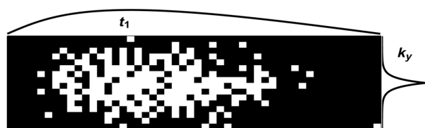
Figure 4. Non-uniform under-sampling (NUS) mask used to under-sample the k_y - t_1 plane 4× in Figs 8 and 9.
