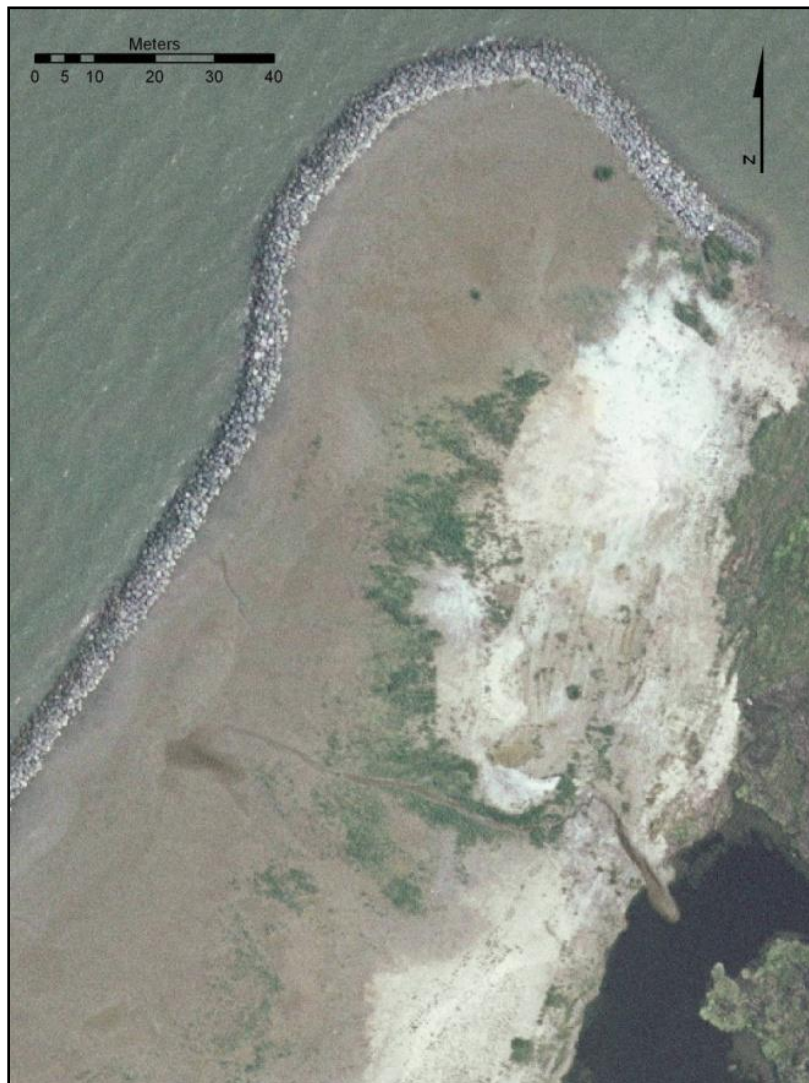
Figure 6. Northern end of Barren Island where stone breakwater was constructed in 2003, dredged material was placed, and planted with Spartina (photo August 2005).
