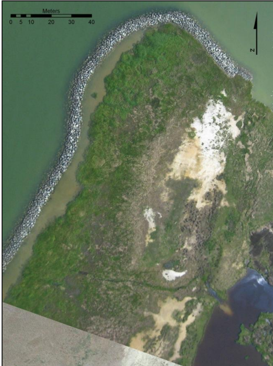
Figure 9. Spartina growth on dredged material placed behind stone breakwater on northern end of Barren Island in August 2008, 3 years after planting.
