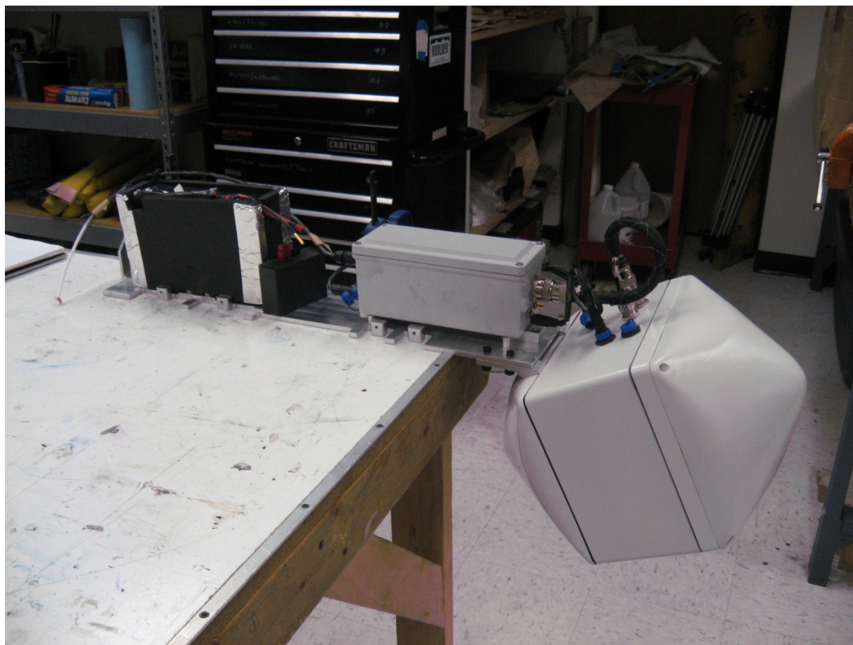
Figure 3a: CULPIS-X in CU-Boulder Lab. Sensor package on right, data acquisition box in middle, battery on left
