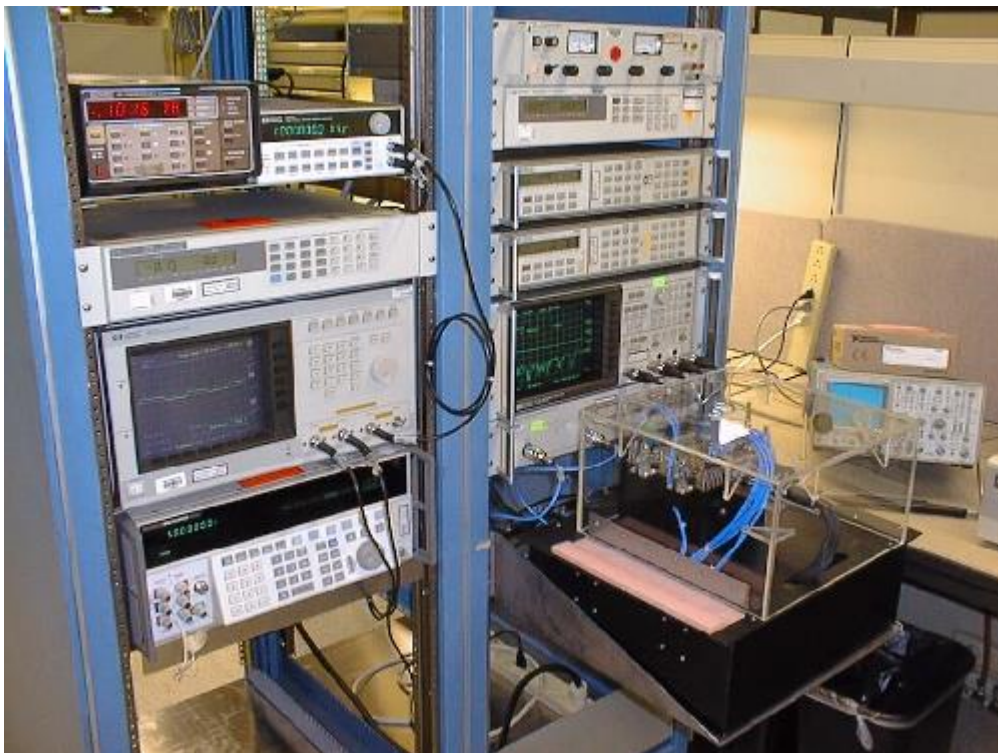
Figure C-1. CCAMTF Automated Test Set
