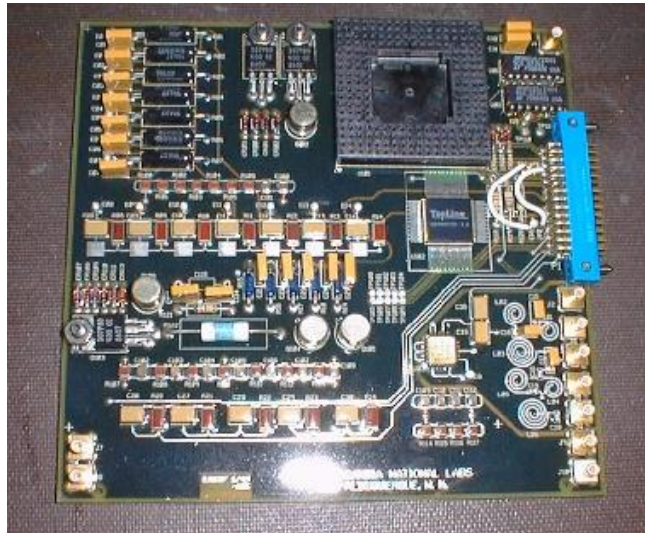
Figure B-6. LRSTF Functional Test Board
