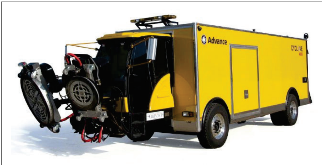
Figure 5. Cyclone 4006 rubber removal system.
