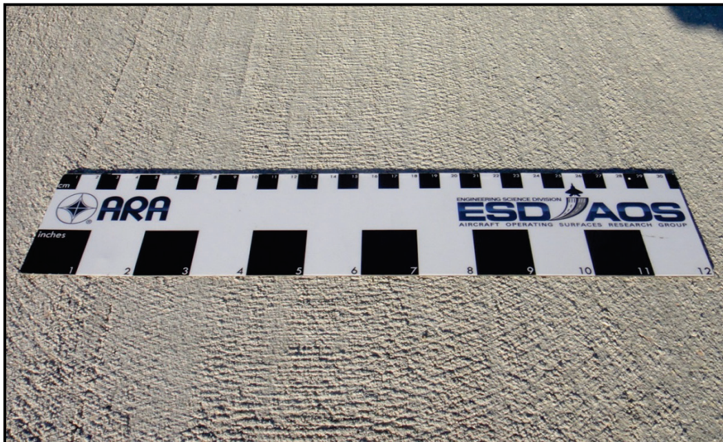
Figure 76. SH8000R PCC etching.
