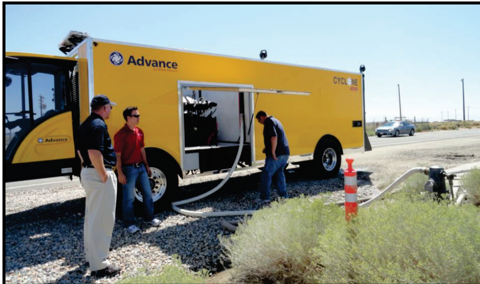
Figure 67. Cyclone 4006 filling with water at hydrant.
