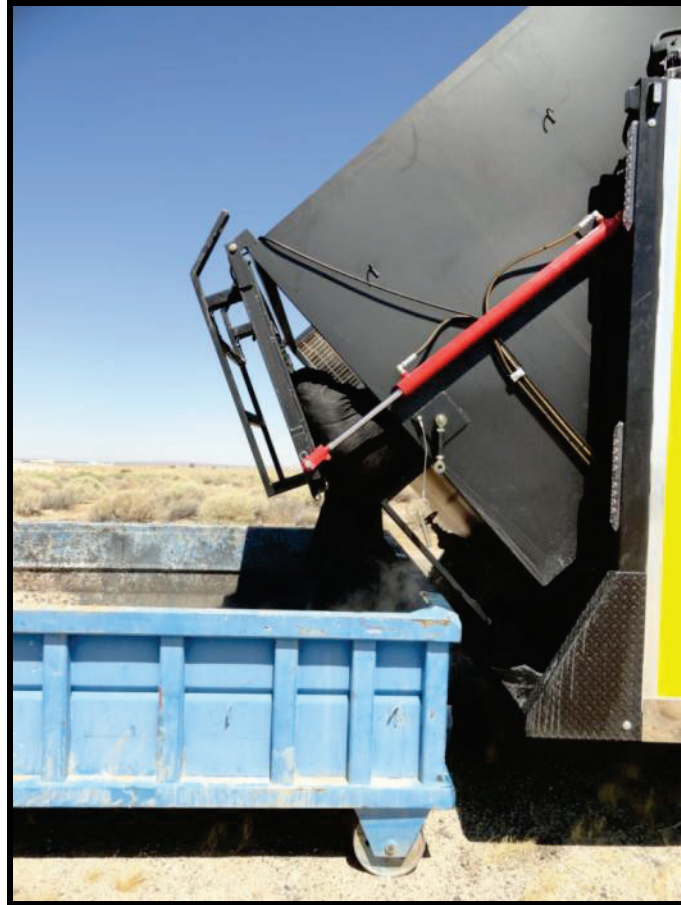
Figure 70. Cyclone 4006 dumps solids.
