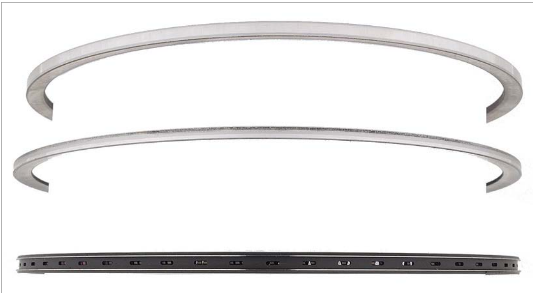
Figure 57. Ring Pack, Cylinder #4
