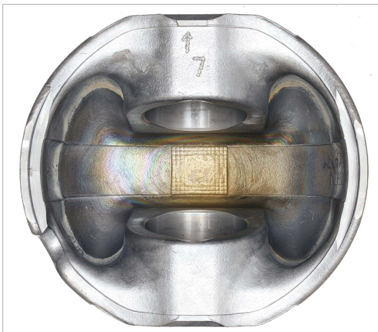
Figure 49. Piston Undercrown, Cylinder #7
