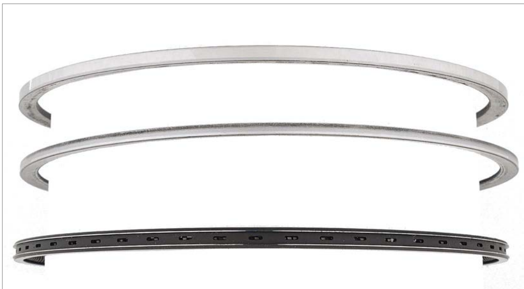
Figure 54. Ring Pack, Cylinder #1
