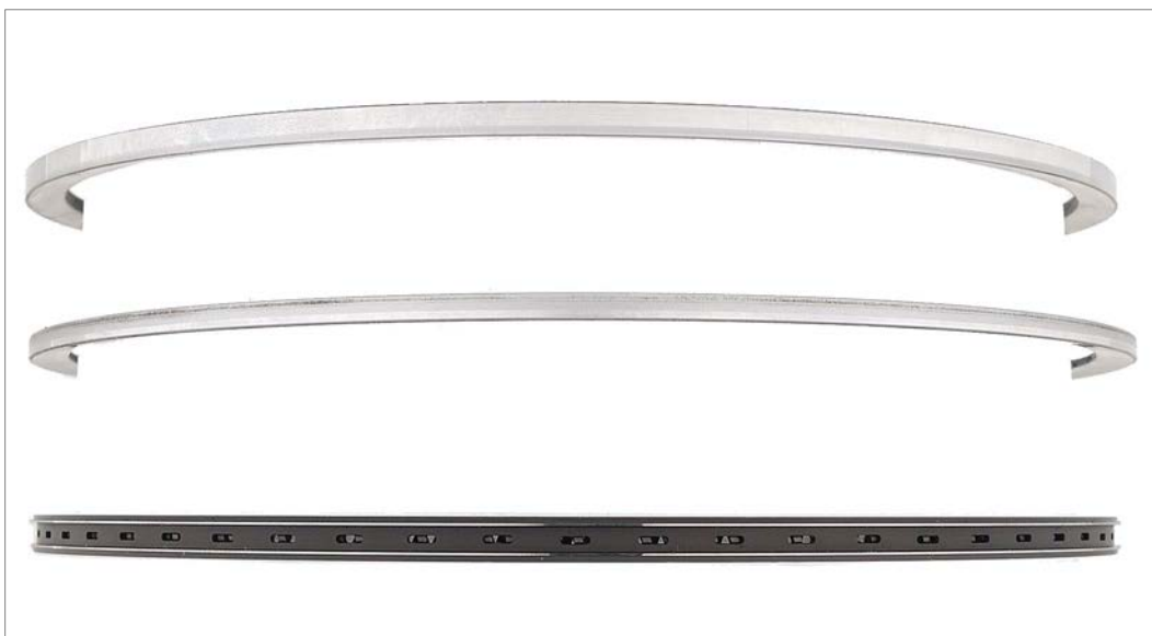
Figure 61. Ring Pack, Cylinder #8
