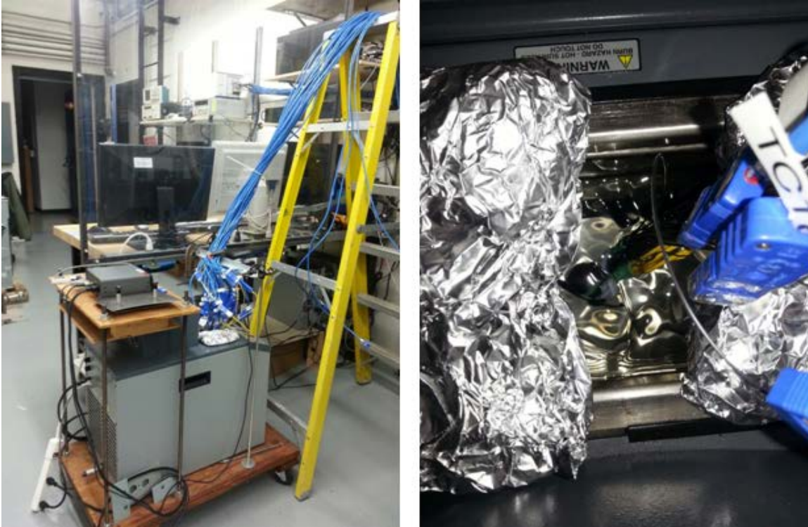
Figure I-1 Calibration Setup (Left) Close Up of Thermocouples in Bath (Right)
