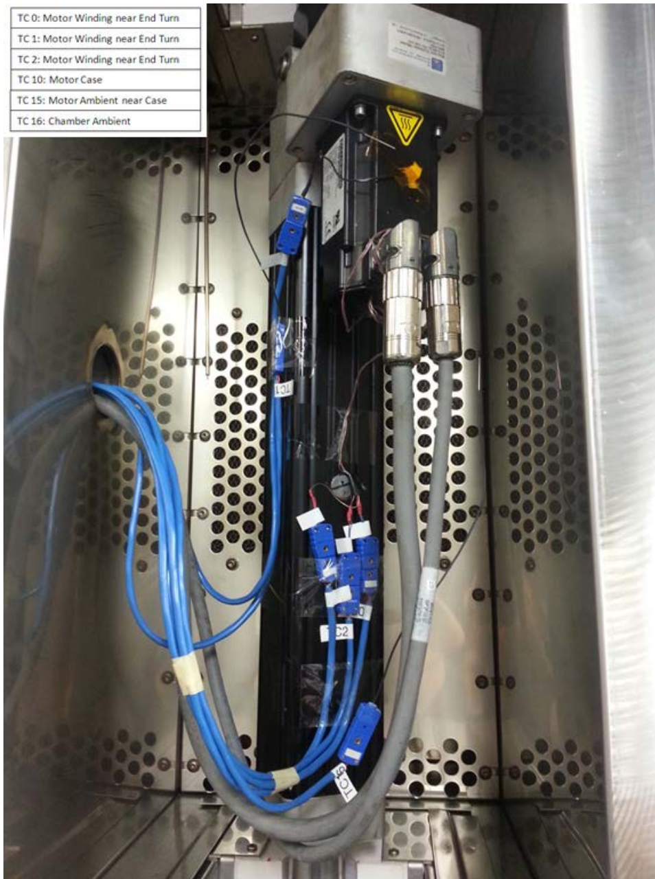
Figure F-8 Thermocouples embedded in motor and within environmental chamber
