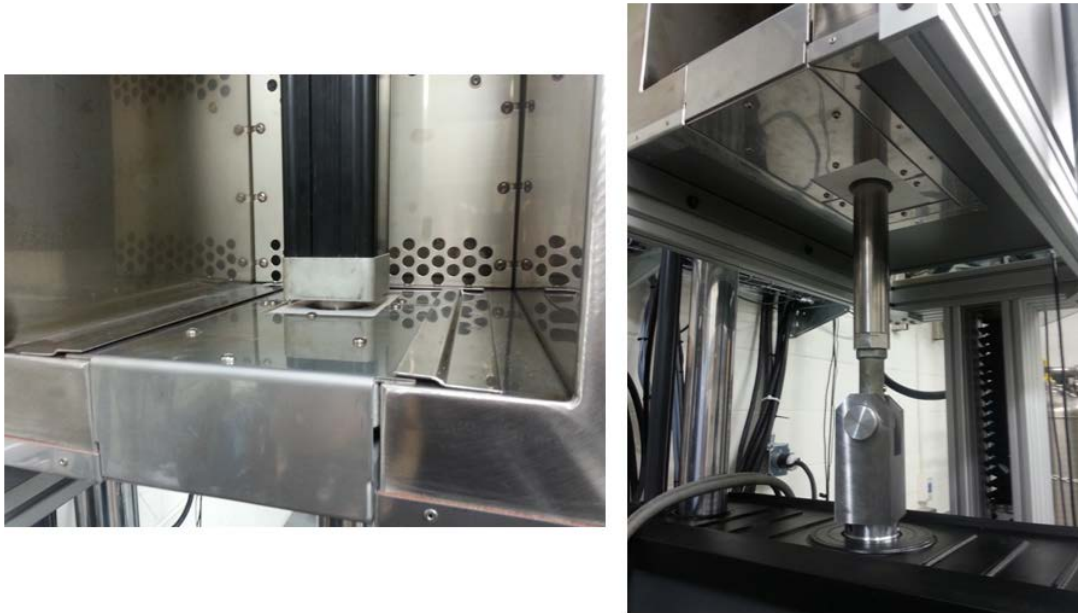
Figure A-3 Environmental Chamber outfitted with Modified U-Plugs—Lower Section
