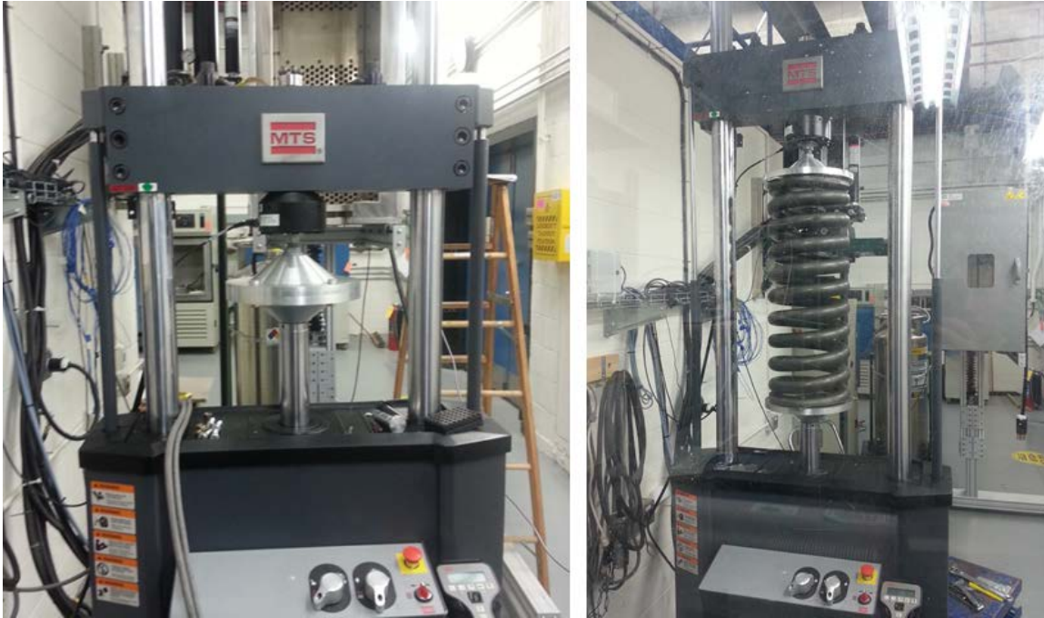
Figure 4.10 Hydraulic Press Characterization Setup (Aluminum Plates)—Left and (Spring)—Right
