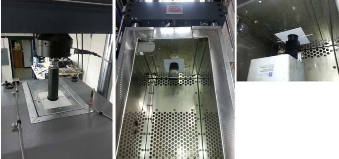
Figure A-2 Environmental Chamber outfitted with Modified U-Plugs—Upper Section
