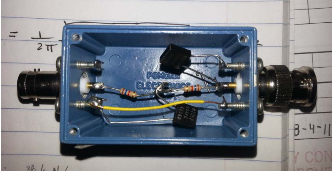
Figure 4.5 2 nd Order Low Pass Filter for Mechanical Measurements
