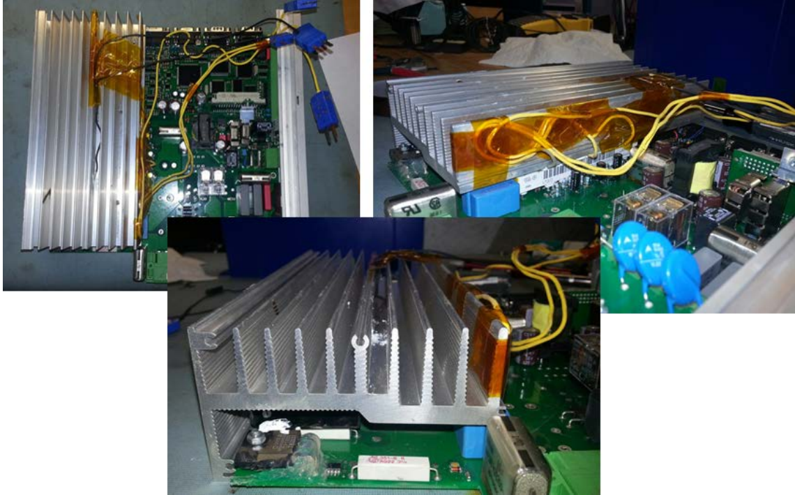
Figure F-4 Thermocouples embedded in Drive 1
