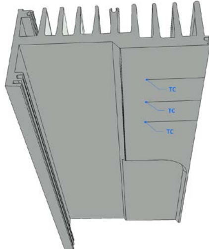
Figure F-3 Underside of heat sink with placement of thermocouples shown
