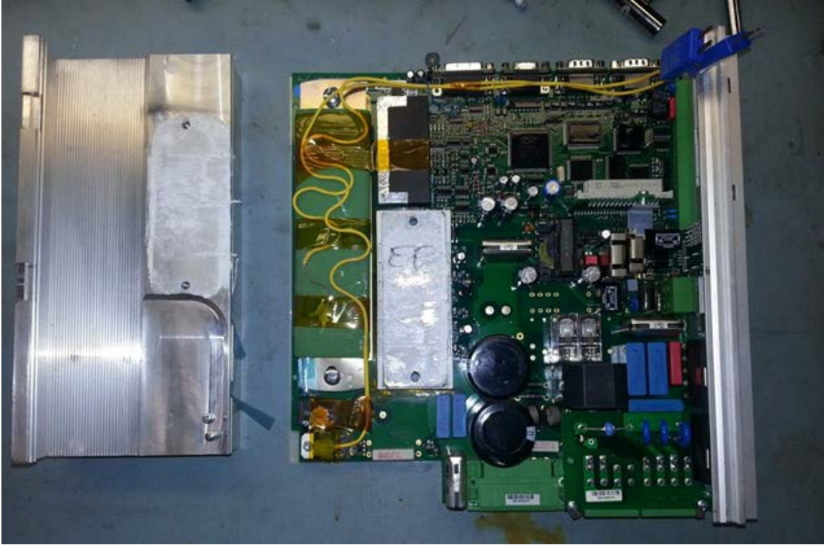
Figure F-6 Thermocouples embedded in Drive 2
