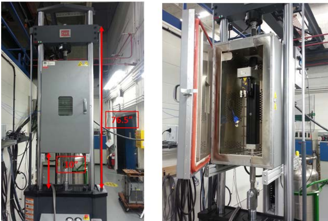
Figure A-4 Environmental Chamber-Hydraulic Press Configuration
