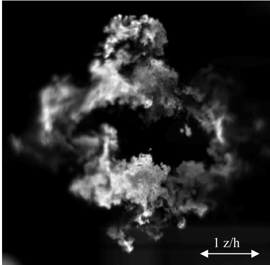
Figure 9 – Sample of instantaneous cross-stream image for Mach 1.3 rectangular jet.
