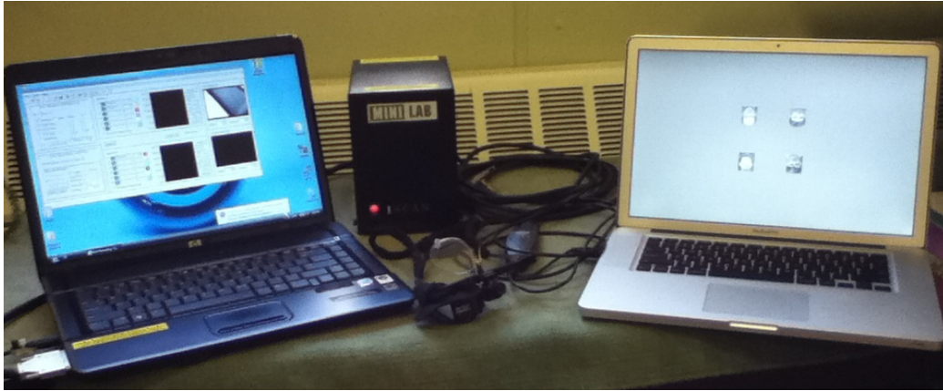
Figure 3: The complete hardware kit. The data-collection laptop is on the left, the video-presentation and data analysis laptop is on the right. The eye-tracker is in the center, its electronics (MiniLab) is in the back, the head-mounted eye cameras and IR mirror attached to a safety-goggle frame are in the front. The Keyspan serial-USB adapter connecting the eye-tracker to the data-analysis laptop can be seen in the center.
