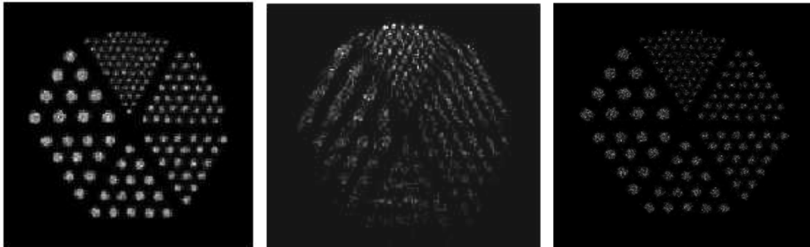
Figure 7. Preliminary 3D PET reconstructions of phantom shown in Fig. 6. Left: ring-ring coincidences only. Center: probe-ring coincidences only. Right: composite reconstruction. Although the composite reconstruction in this case fails to show significant improvements, there are two significant issues. First, the resolution of the PET ring was nearly as high as could be supported by the pixel size in the reconstruction; and second, significantly more iterations are required for convergence in combined dataset.
