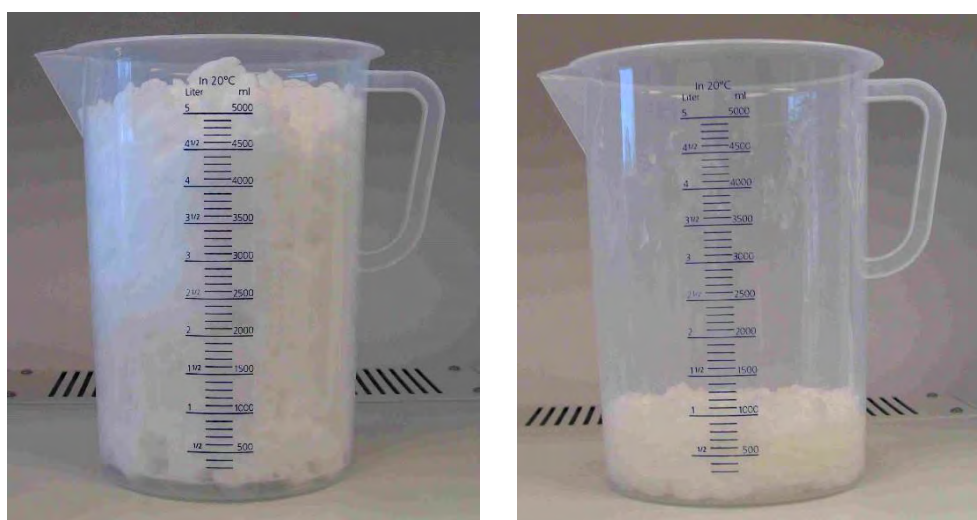
Figure 25. Alginate foam as produced (left) and after mechanical stress (right).
