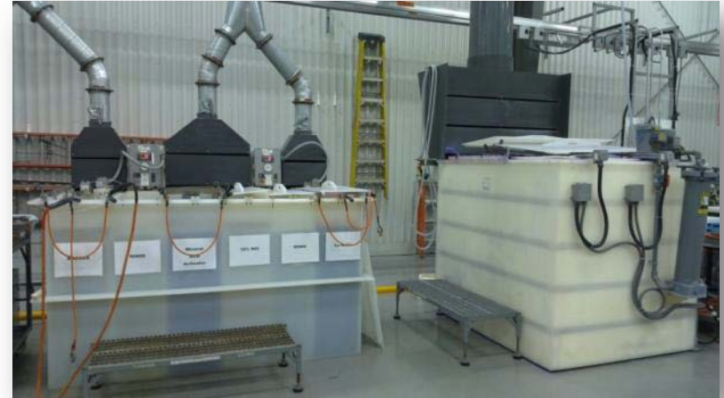
660 gal nCoP Plating tank at Integran
