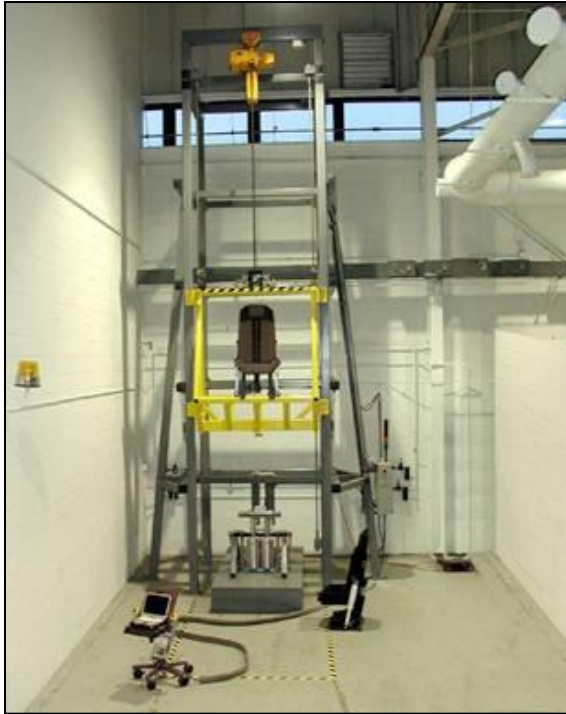
Vertical drop tower test fixture
