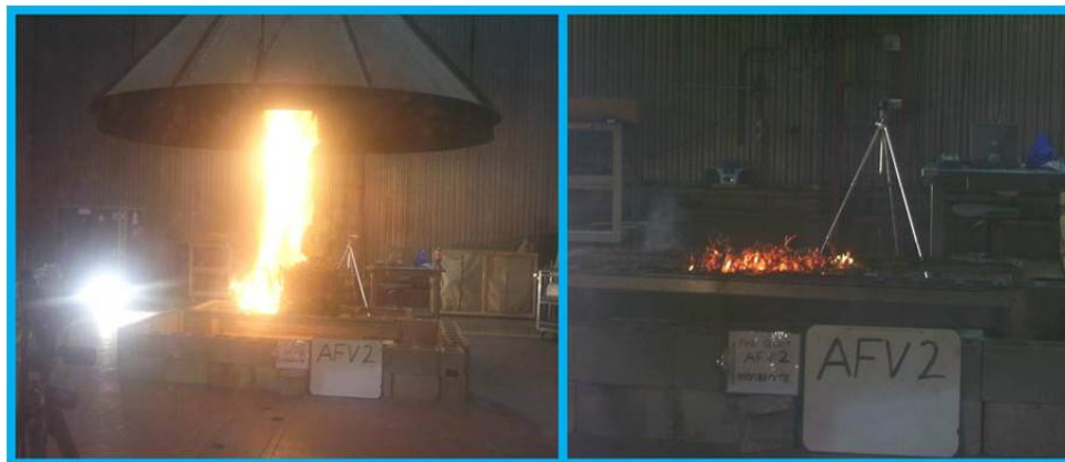
Figure 2.4 Evidence of the capability to realistically simulate fires at the FSL combustion facility for the flaming and smoldering phases of Vandenberg AFB fuels
