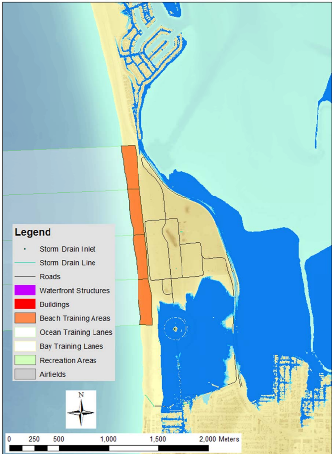
Figure 5-124. Detailed view of inundation and flooding for the 2.0 m SLR bay-exposure scenario at SSTC South. The blue shaded zones represent week (dark blue), year (medium blue) and century (light blue) return periods.
