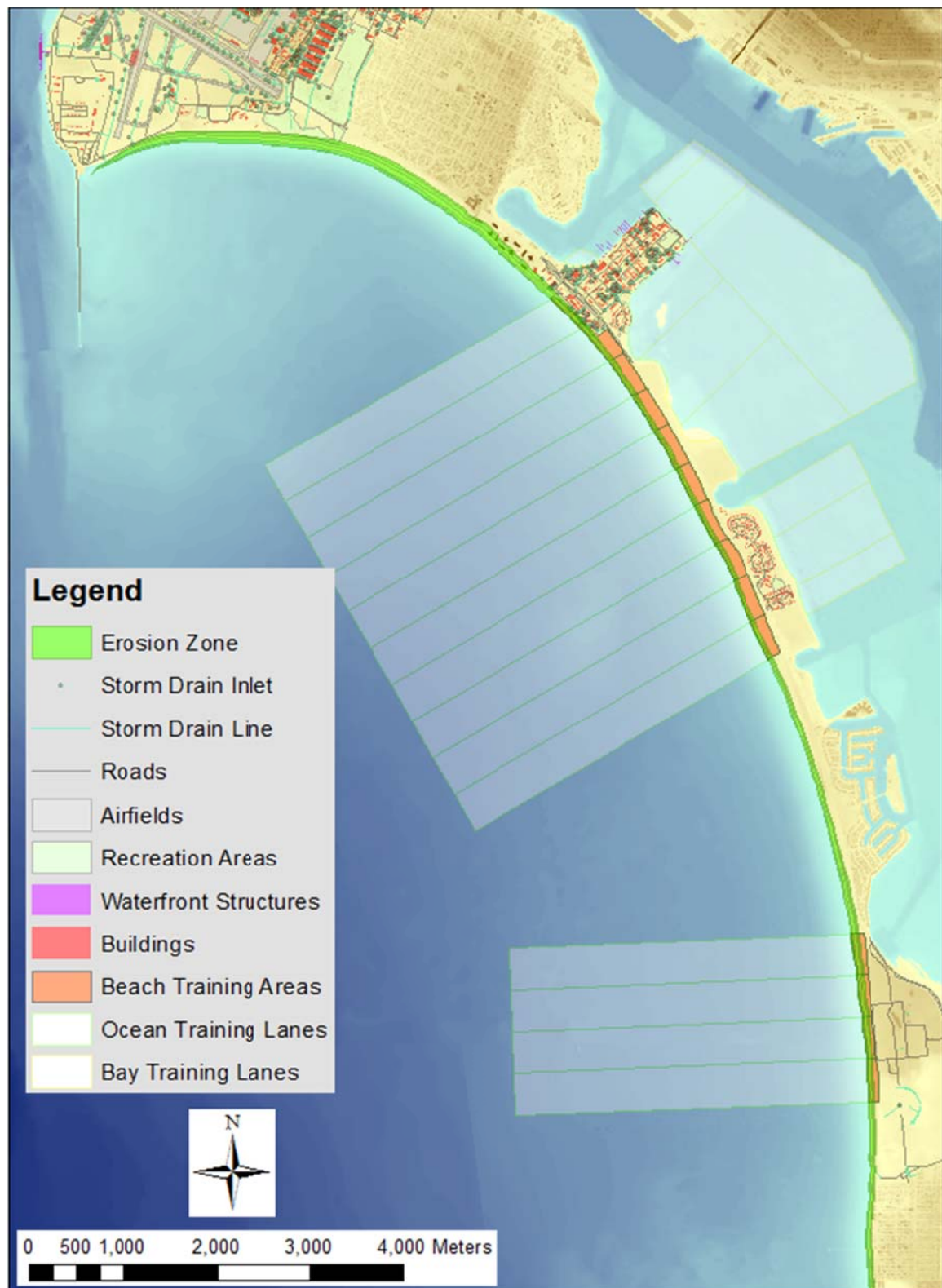
Figure 5-59. Erosion footprint for the baseline (SLR=0 m) scenario at NBC. The overall green shaded band spans the 100 year return period wave condition from the YGOR model, and the fine grey lines indicate the shorter return periods ranging from week to decade.
