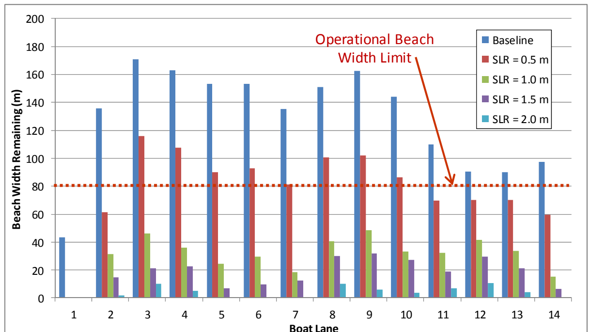
Figure 5-227. Beach width remaining by training lane at SSTC for the monthly return period flood event.
