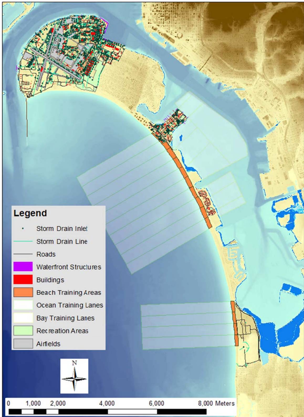
Figure 5-113. Inundation and flooding for the baseline (SLR=0 m) bay-exposure scenario at NBC. The blue shaded zones represent week (dark blue), year (medium blue) and century (light blue) return periods.
