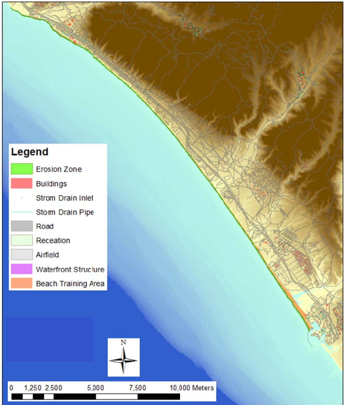
Figure 5-75. Erosion footprint for the baseline (SLR=0 m) scenario at MCBCP. The overall light green shaded band spans the 100 year return period wave condition from the YGOR model, and the fine grey lines indicate the shorter return periods ranging from week to decade.
