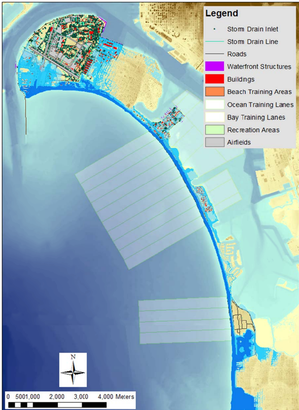
Figure 5-92. Inundation and flooding for the SLR=1.0 m scenario at NBC. The blue shaded zones represent week (dark blue), year (medium blue) and century (light blue) return periods.
