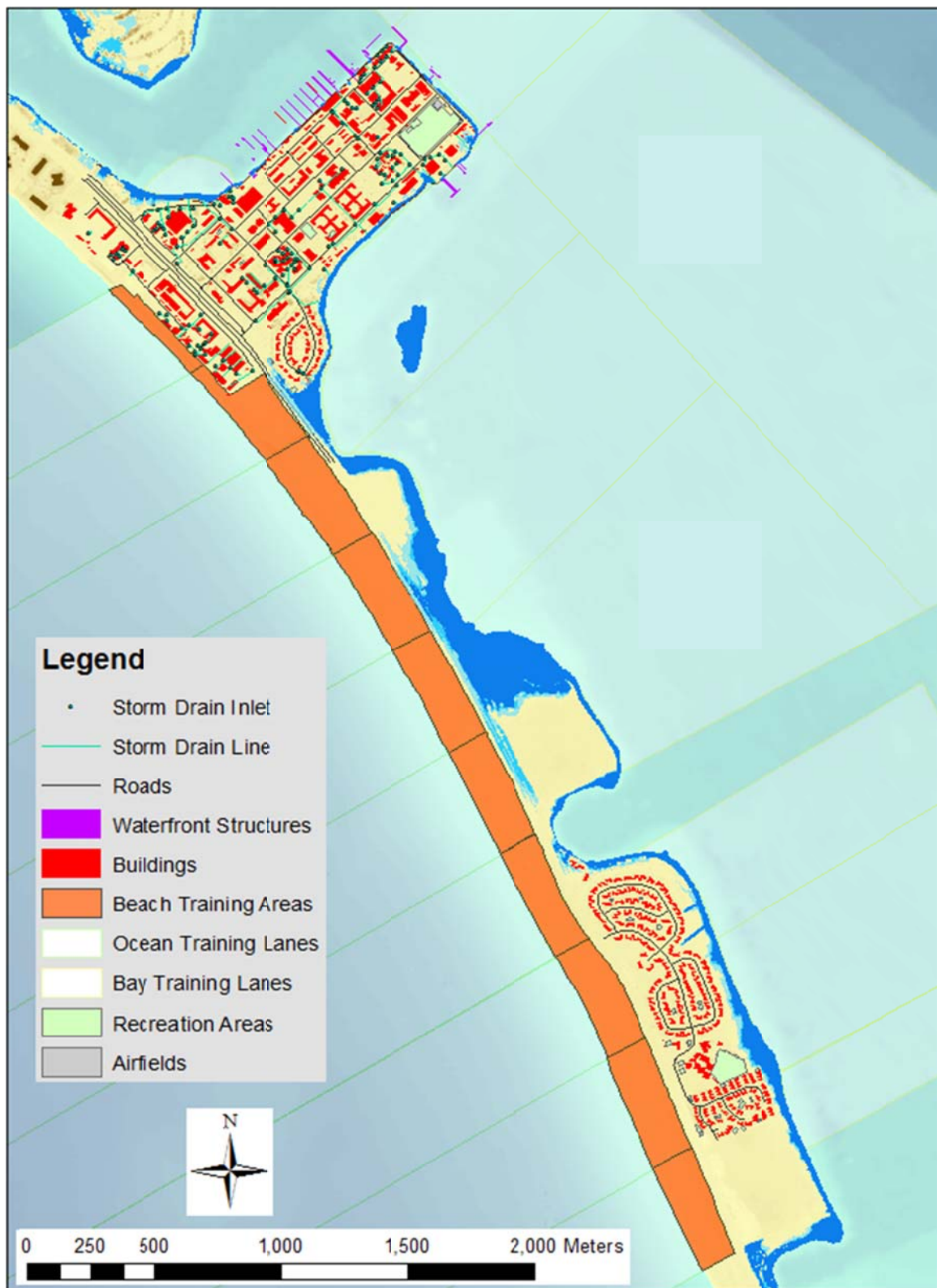
Figure 5-119. Detailed view of inundation and flooding for the 1.0 m SLR bay-exposure scenario at NAB/SSTC North. The blue shaded zones represent week (dark blue), year (medium blue) and century (light blue) return periods.
