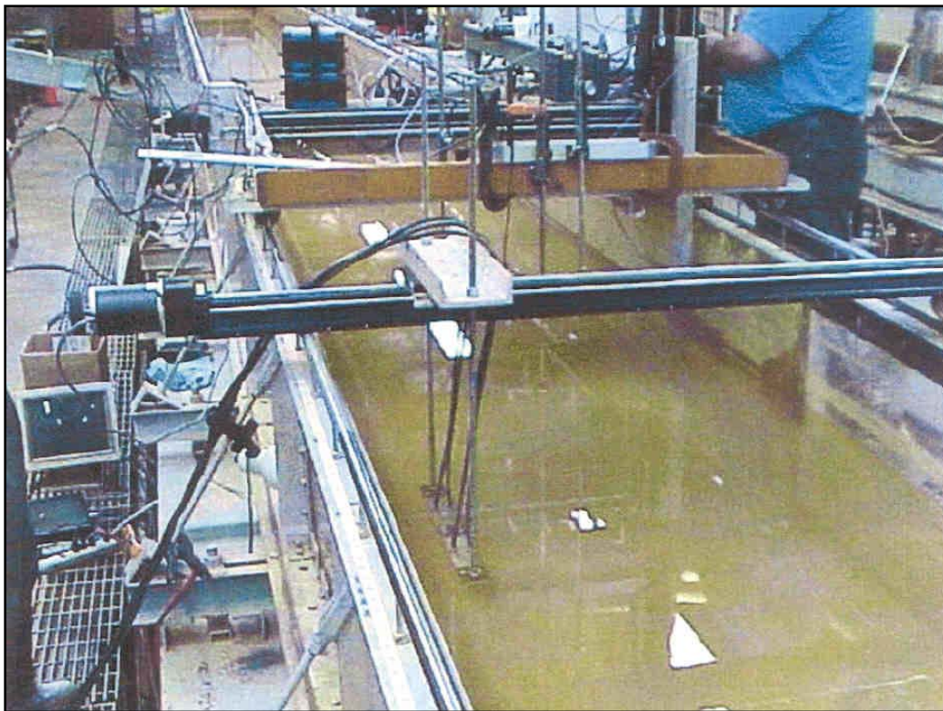
Figure 8. Seatek acoustic sensors mounted on the automatic traversing mechanism in test flume.
