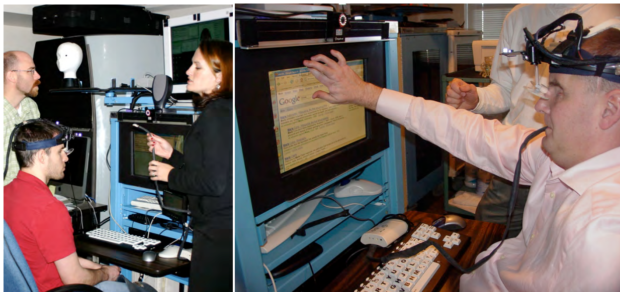
Figure 4: Direct computer tactile (BrainPort®) interface demonstrations. left , participant prepares to use eye/head tracking apparatus to determine point of gaze despite the users' prosthetic eyes. The software determines if the participant is looking at the screen and returns a 100-200 pixel sample of the screen image. The user intuitively controls zoom level by leaning either toward or away from the screen. Looking down automatically selects a gaze directed subsample of the video image from the head mounted camera (allowing the user to find keys on the keyboard). right , When the user touches the screen, the subsection of the screen image underneath the fingertip is presented to the tongue instead.
