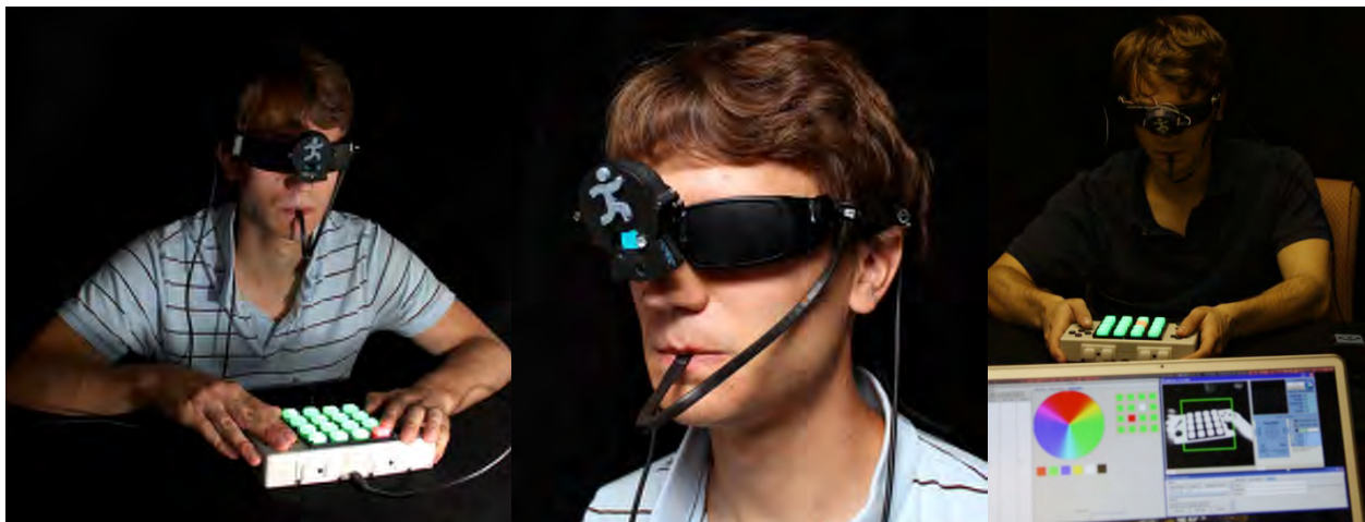
Figure 6: Research staff (using BrainPort®) changing filter (black disk mounted to glasses) with Playstation3 game controller buttons to identify color of illuminated button pad.
