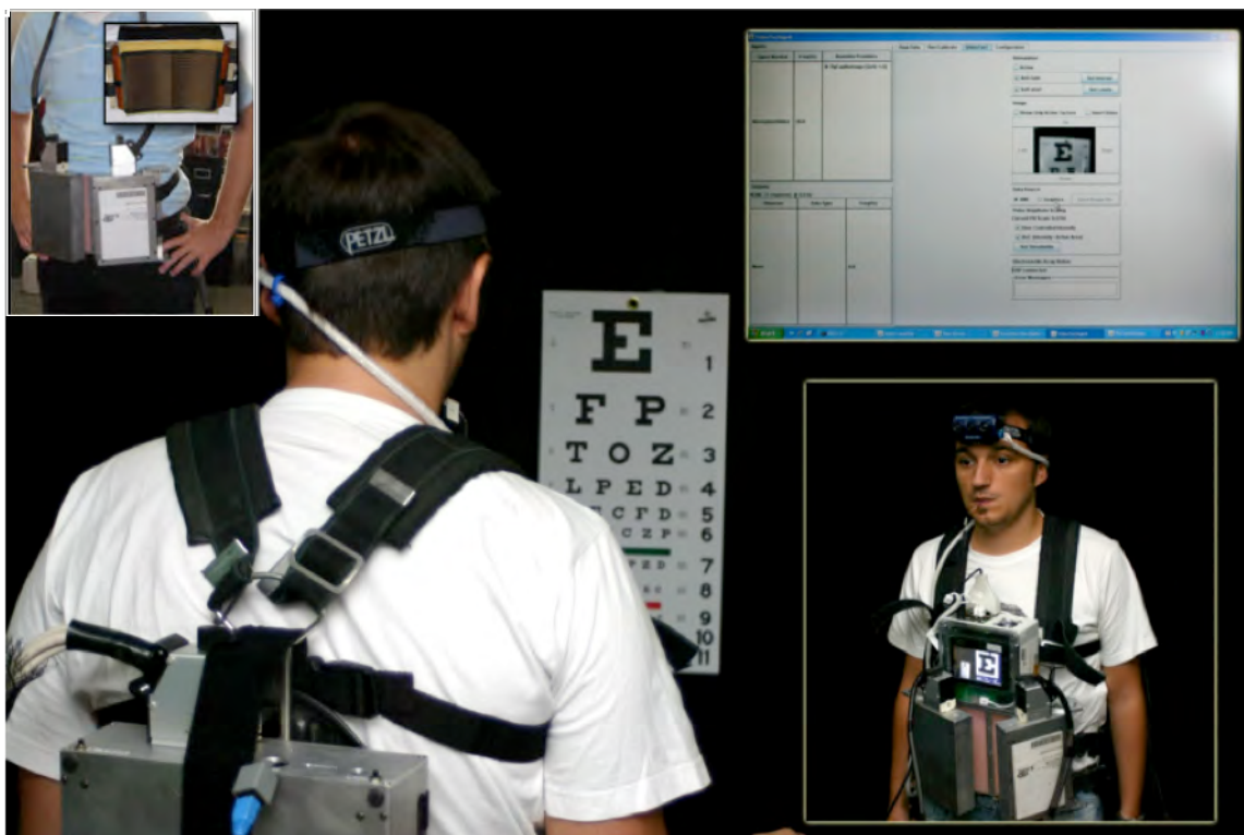
Figure 5: Initial mock up of ACMI-VAS for foveal and paracentral vision substitution. Image (upper right inset) presented on the VideoTact (upper left inset) is zoomed in less than the BrainPort ® image zoom level (center display of lower right inset) to provide a slightly wider field of view. The physical size of the components has been reduced significantly and control of the combined technologies has also been simplified using IHMC's AMI architecture.
