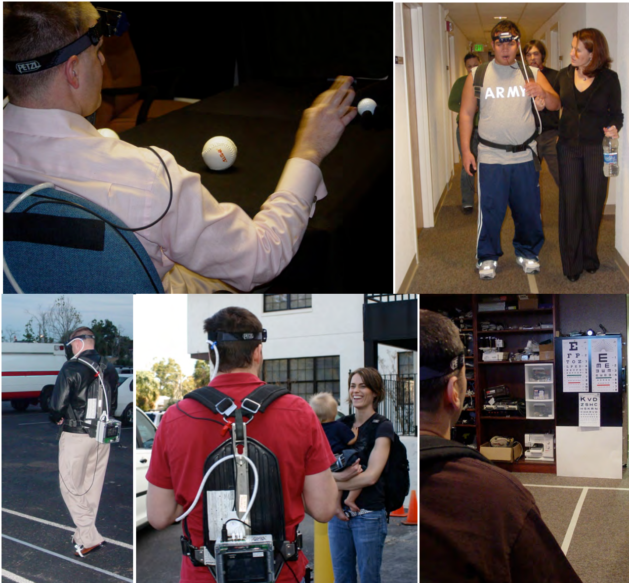
Figure 3: Initial BP-WAVE II activities performed during technology demonstrations with recently blinded servicemembers. left to right, top to bottom , Catching balls, navigating office spaces, locating open parking stalls, noticing infant's hair, and reading eye charts to 20/80 ( images used with permission ).
