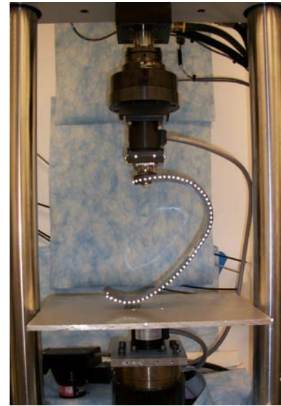
Figure 2. Running-specific prosthesis (Ossur Flex-Run) setup in the MTS machine.
