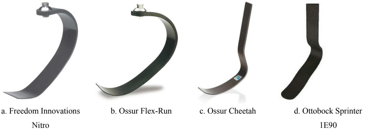
Figure 1. Prostheses used for mechanical testing.
