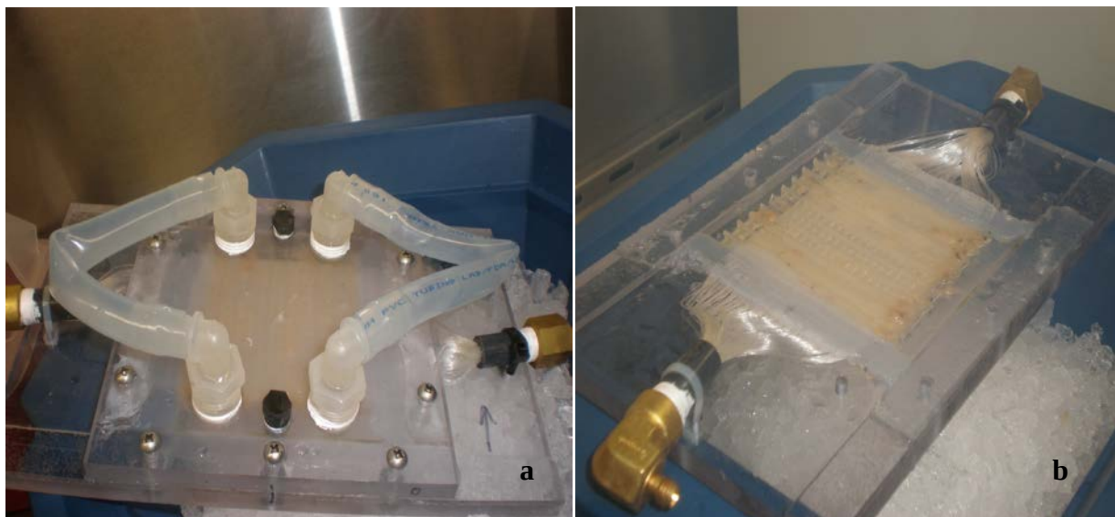
Figure 1a Side reactor shipped to ASU. 1b Biomass development on the surface of fibers in the side reactor.
