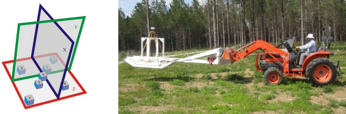
Figure 5-1. Schematic and photo of the MetalMapper as used at former Spencer Range
