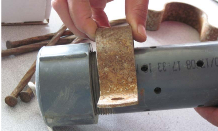
Figure A3. Fasteners used to install the sensors.
