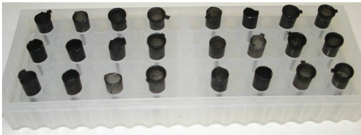
Figure 8. Test spore tubes recovered from explosion chamber after detonation
