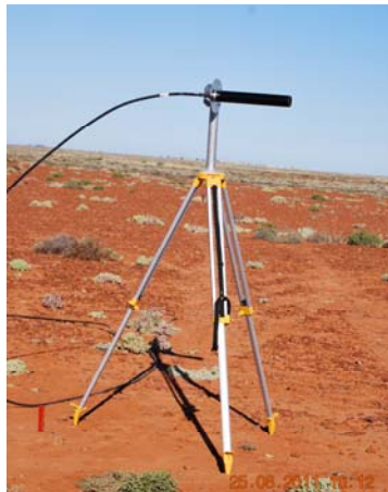
Figure 7: Transmitter site with a helix antenna mounted on a tripod for Scenario 2
