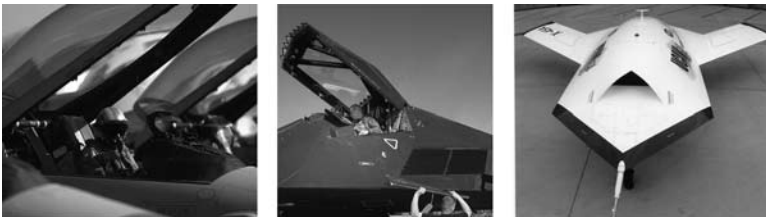
Figure 7. Efforts to reduce RCS: gold canopy, saw-tooth edges, raised engine nacelle. (Photos courtesy of US Air Force.)
