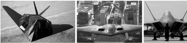
Figure 6. Efforts to reduce RCS: mesh screens, raised nacelles, canted tails. (Photos courtesy of US Air Force.)
