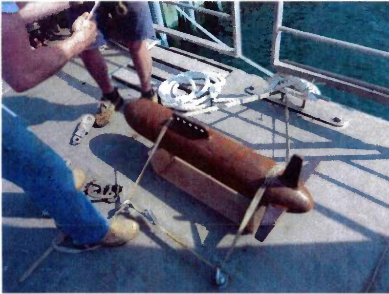
Figure 10: 250 kg towed vehicle to stabilize the end of the towed tether with fairings. Stabilization was impossible beyond a speed of 8 knots, due to kiting.
