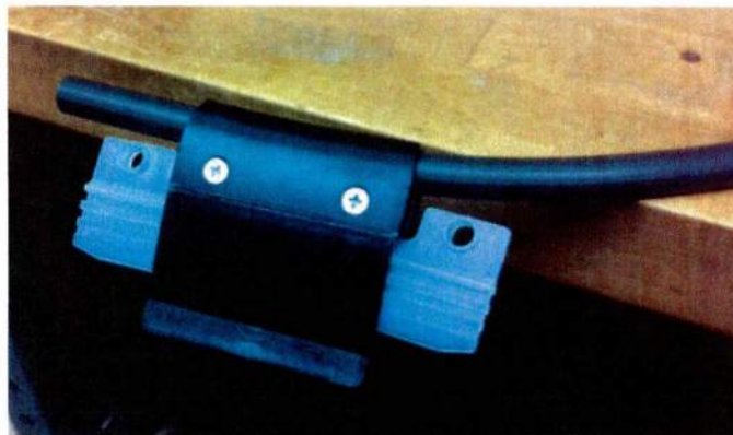
Figure 4: Single fairing on curved rod. Same fairing as in Fig. 2 is on the same rod, but is moved into a region of slight curvature. Fairing is unable to align with gravity.
