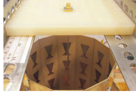
Fig. 5. Coaxial probe for mapping microwave power distribution in the plane of the therapy array (shown in photo without coupling fluid for clarity).
