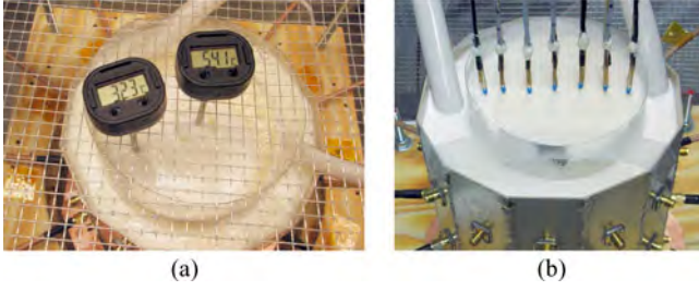
Fig. 4. (a) Initial temperature measurements with digital probe thermometers in 50/50 oil-in-water gelatin phantom with 30/70 oil-in-water cylindrical inclusion. (b) Thermistor array above homogeneous 50/50 oil-in-water gelatin phantom in 60/40 matching fluid.
