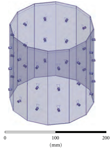
FIGURE 4: HFSS CAD model of the imaging cavity. Twelve panels contain three bow-tie antennas each. The bottom of the cavity is PEC, it is filled with the coupling fluid up to the visible line, and the top surface radiates to air.
